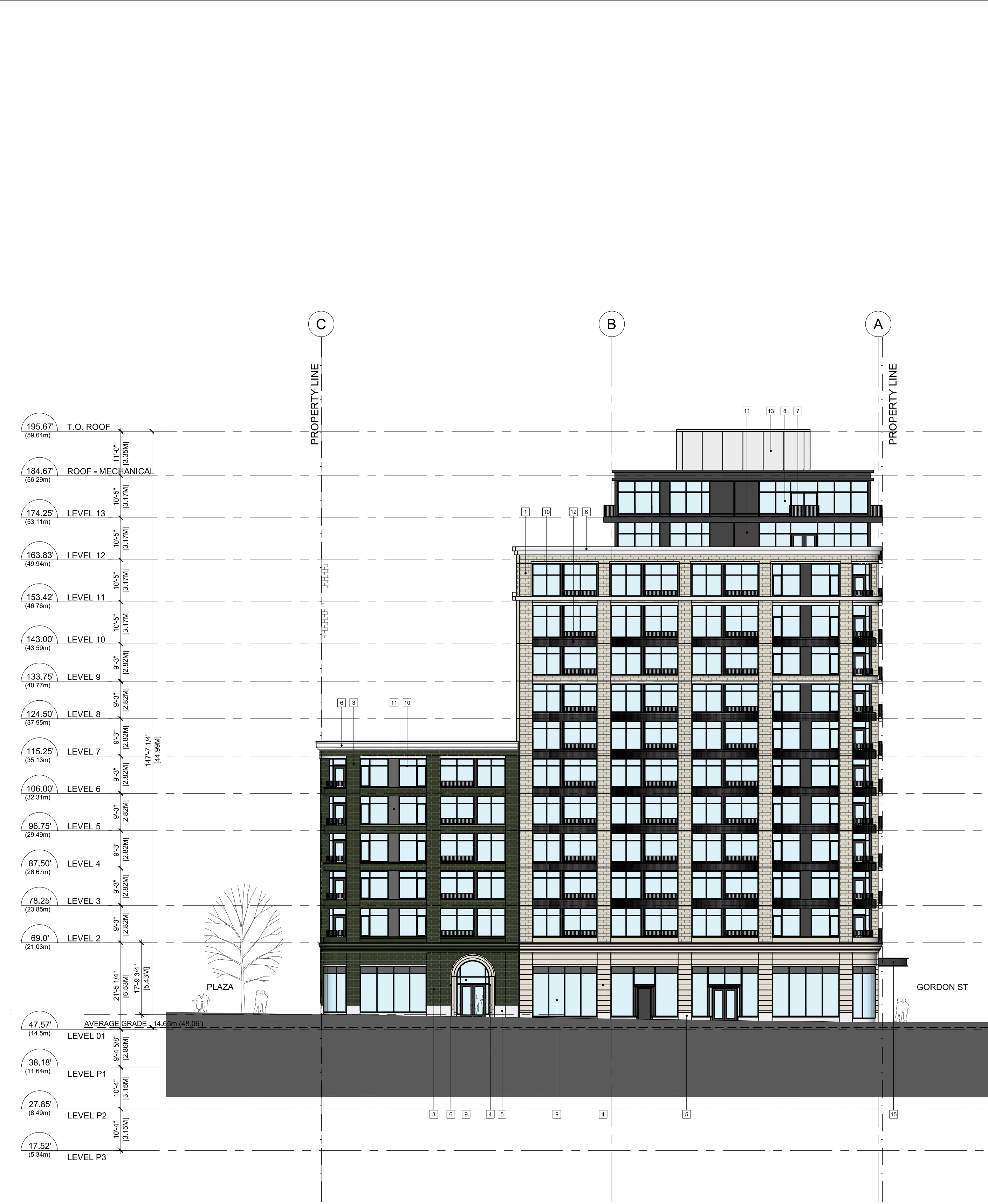
04 BROUGHTON ST ELEVATION (NORTH) 1:250
