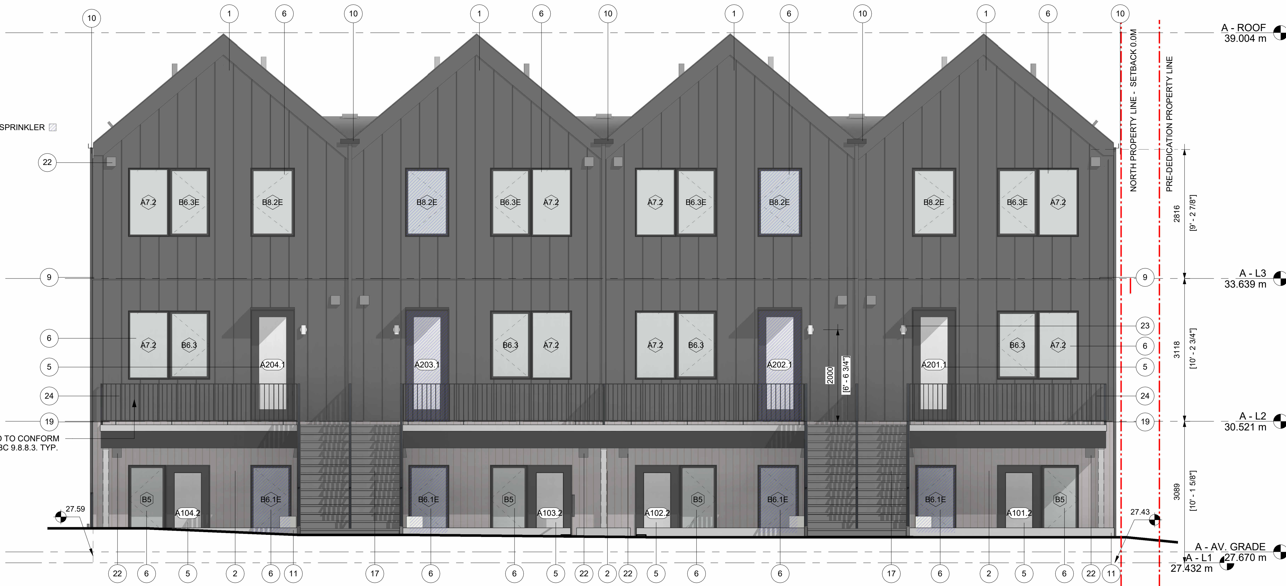
2 BUILDING A EAST ELEVATION A.403 1:50
