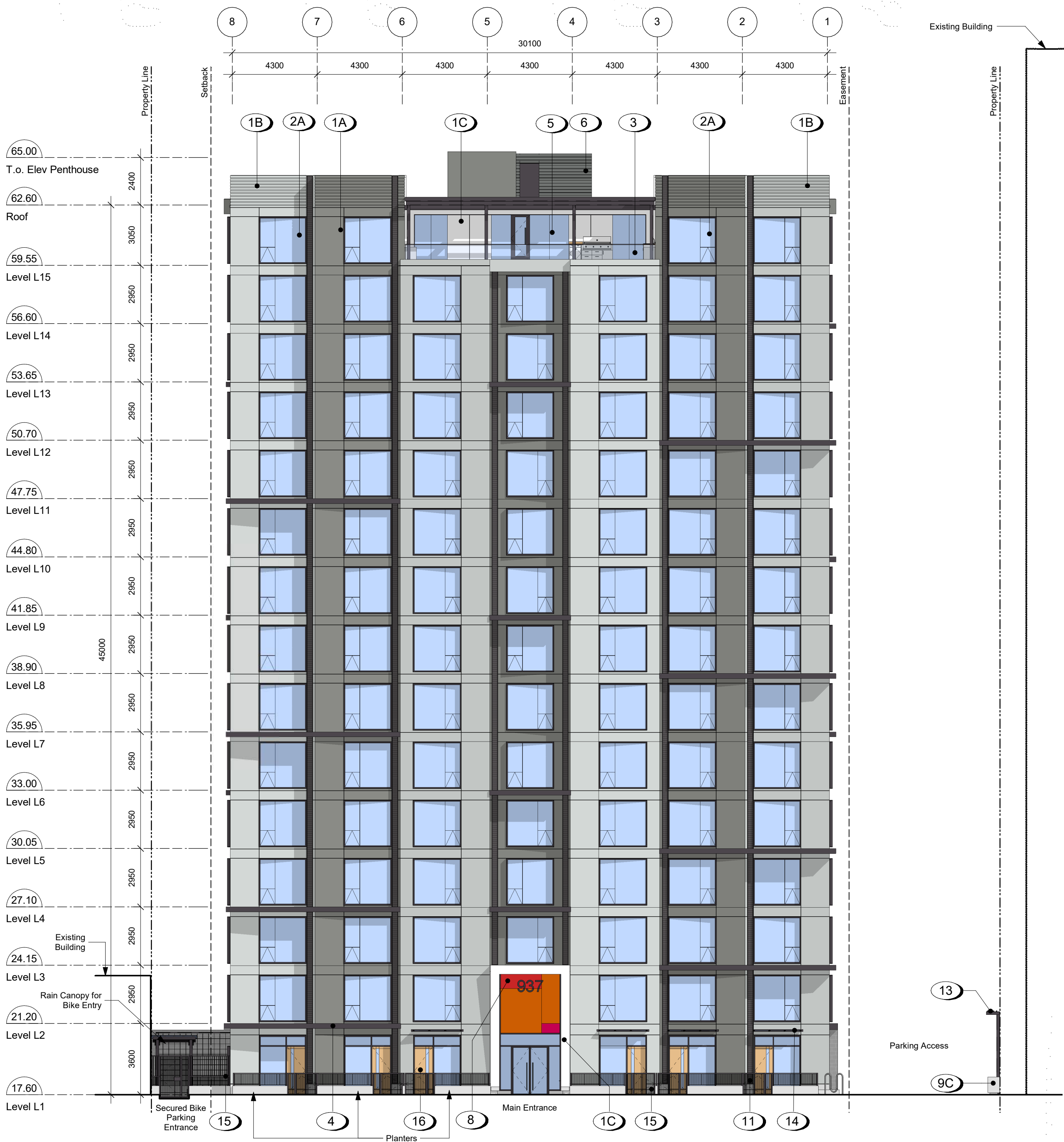
1 Building Elevation - North A301 SCALE: 1 : 150
