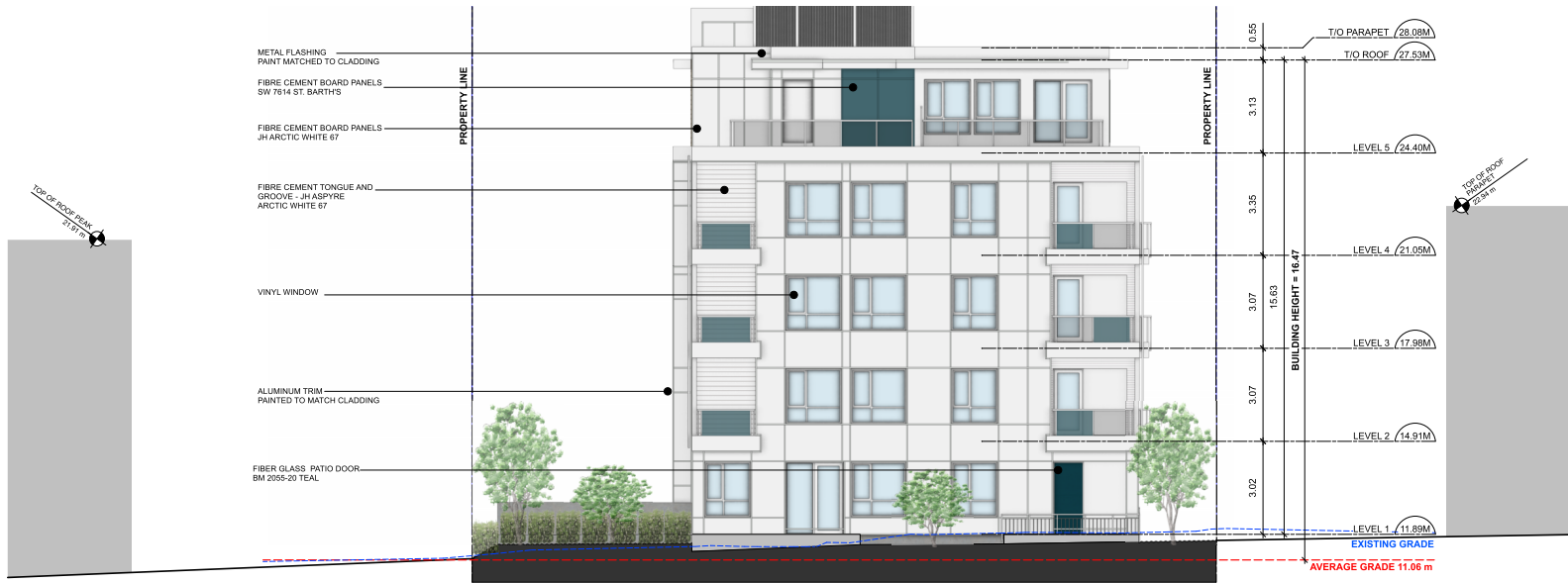
1 SOUTH ELEVATION - REAR FACADE Scale: 1/75
