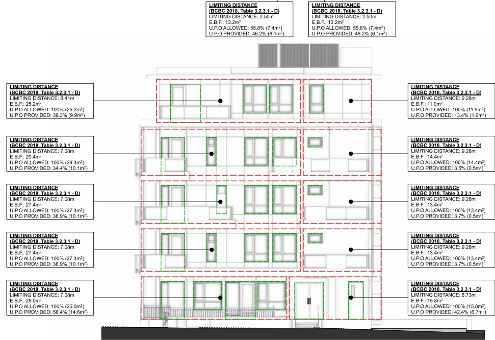
1 NORTH ELEVATION - FRONT FACADE Scale: 1/75
