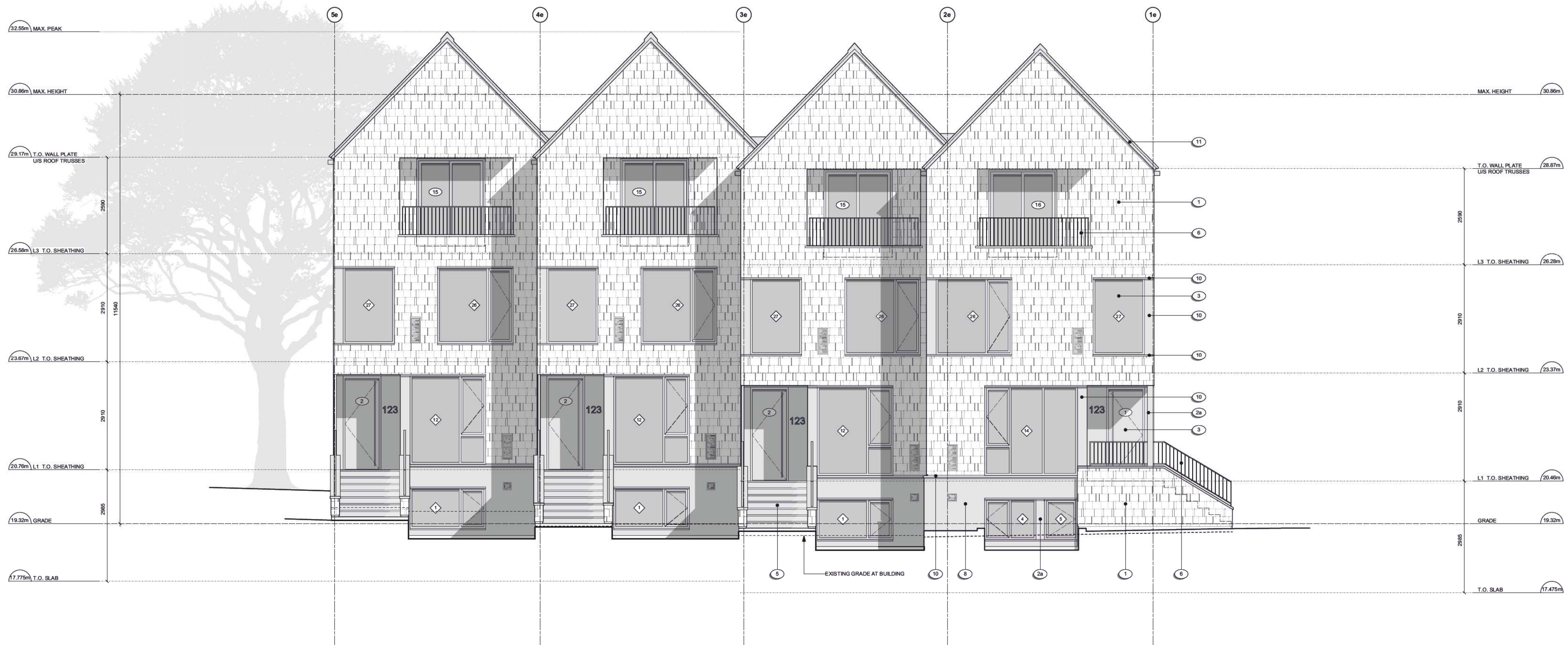
2 East Bldg. - West Elevation Scale: 1:50
