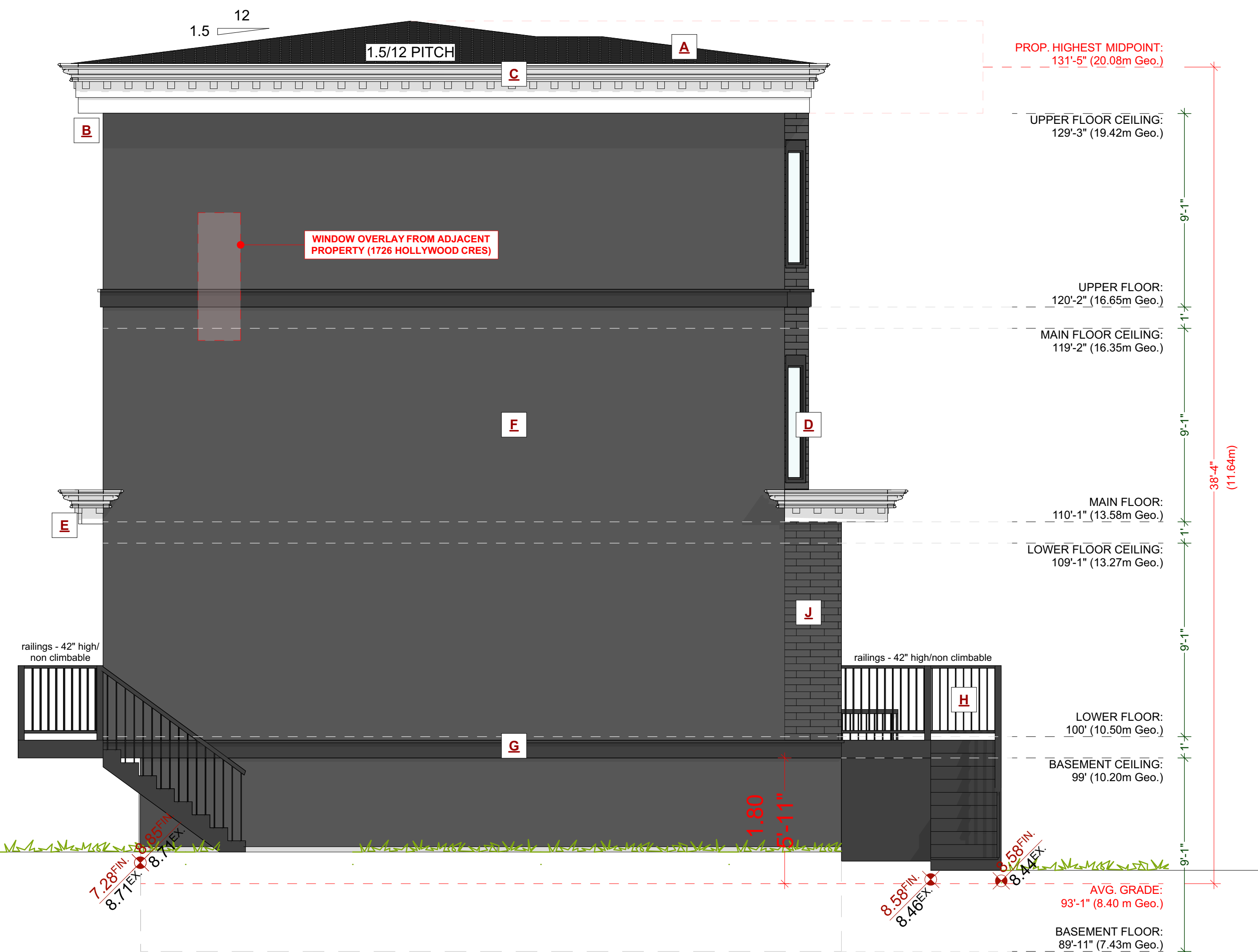
B PROPOSED WEST ELEVATION SCALE: 1/4" = 1' - 0"
