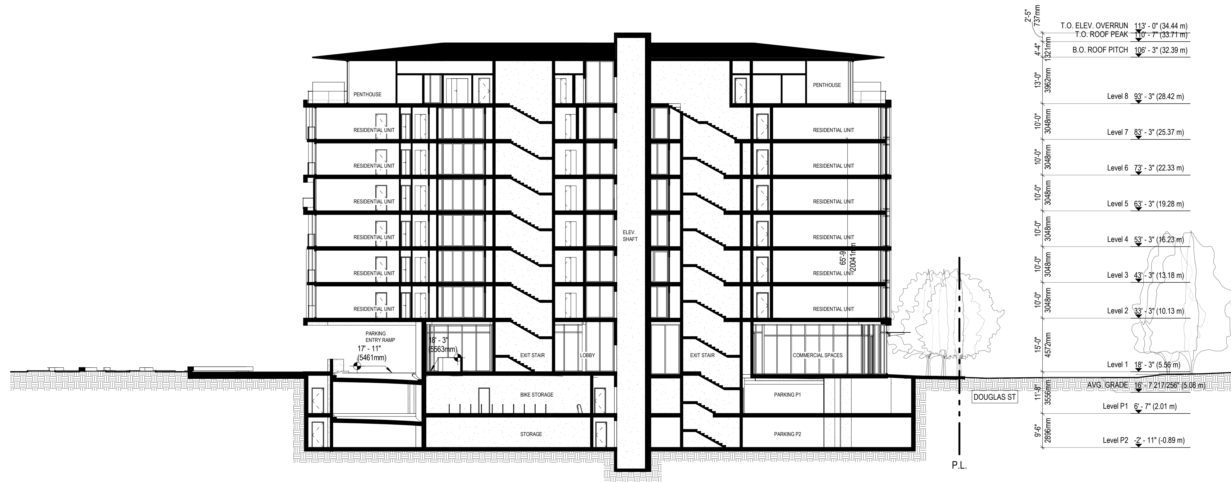
A-A BUILDING SECTION A A2.03
