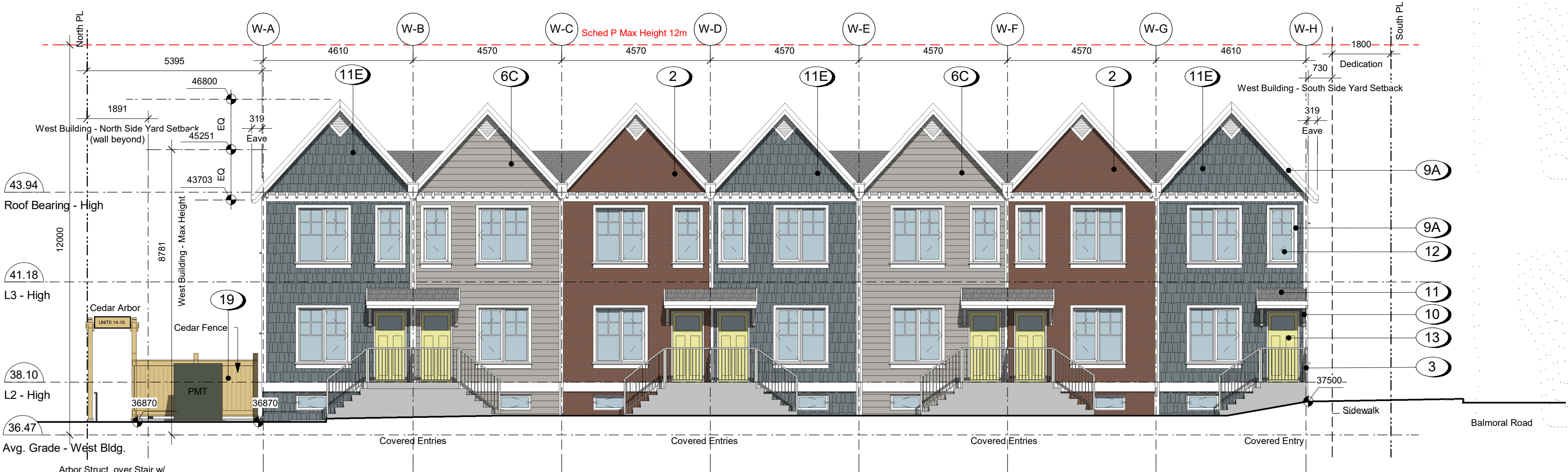
1 West Building - West Elevation A301A SCALE: 1 : 100
