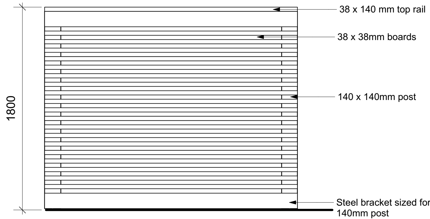
6 1.8m ht. Timber Perimeter Fence Scale: 1:20
