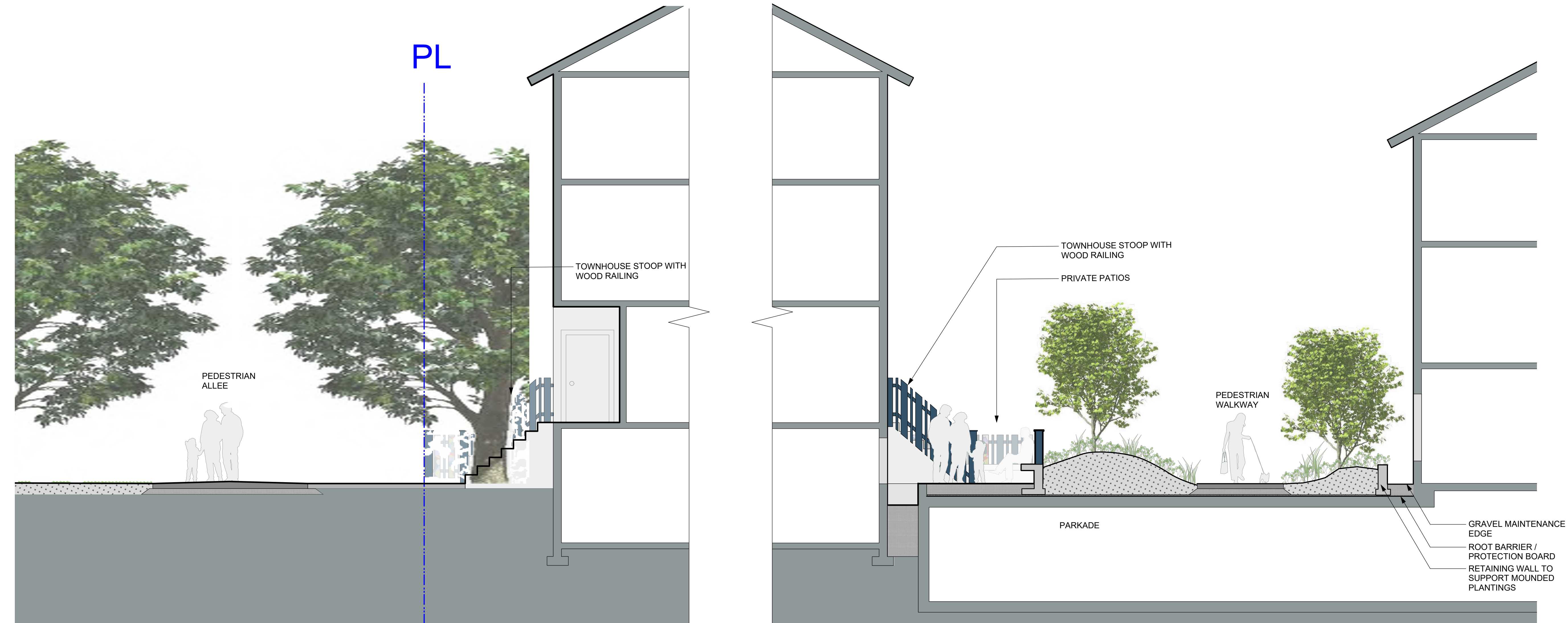
1 Section at Pedestrian Allee and Townhouses Scale: 1:50
