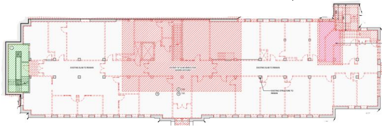
Figure 64: Proposed Outline for Existing Level 1 Slab Demolition. Source: omb Architects + Designers architectural drawings, February 17, 2023. Note the existing west stairwell will be preserved and restored, the NE stair to be demolished for restoration of façade and replaced with new internal exit stair.
