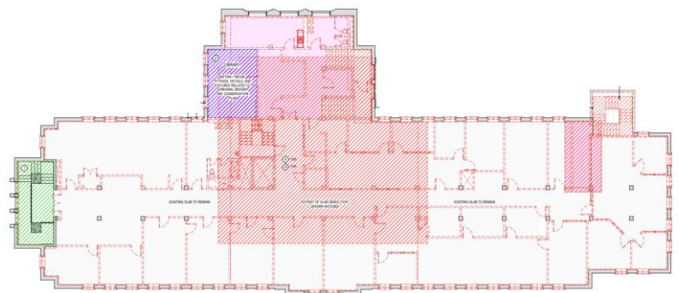
Figure 67: Proposed Outline for Existing Level 4 Slab Demolition. Source: omb Architects + Designers architectural drawings, February 17, 2023. Note the features of the Library, shown in the purple hatched area, will be retained and reused.
