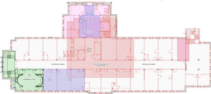
Figure 66: Proposed Outline for Existing Level 3 Slab Demolition. Source: omb Architects + Designers architectural drawings, February 17, 2023. Note the Chairman's Office will be preserved and restored, and features of the Lobby, and the offices of the Secretary and Commissioner shown in purple hatched areas will be retained and reused.
