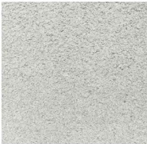
3.1 ▲ TEXTURED REINFORCED FIBER CEMENT PANELS FIRE-HALL EXTERIOR
