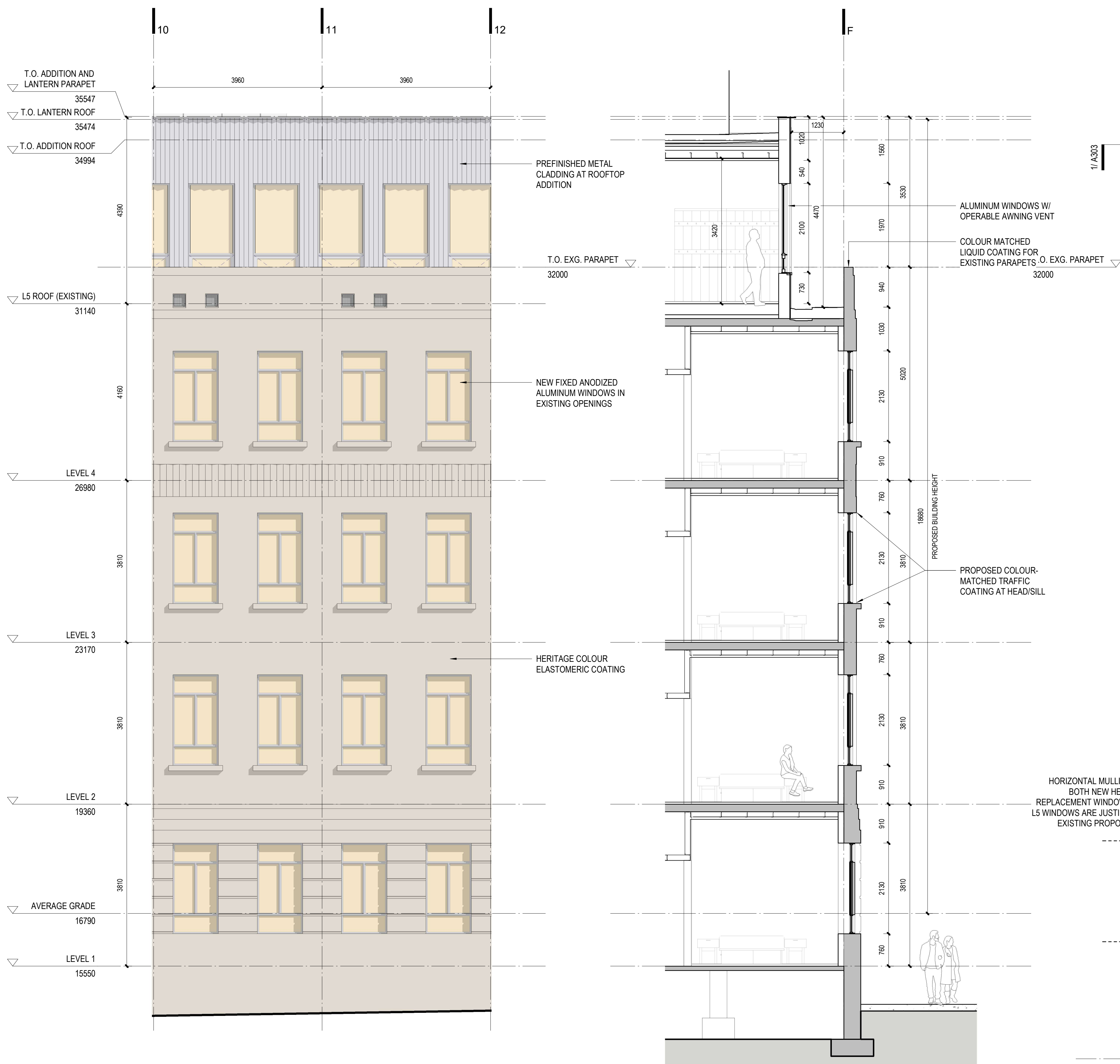
1 TYPICAL BAY - ELEVATION A204 1 : 50
