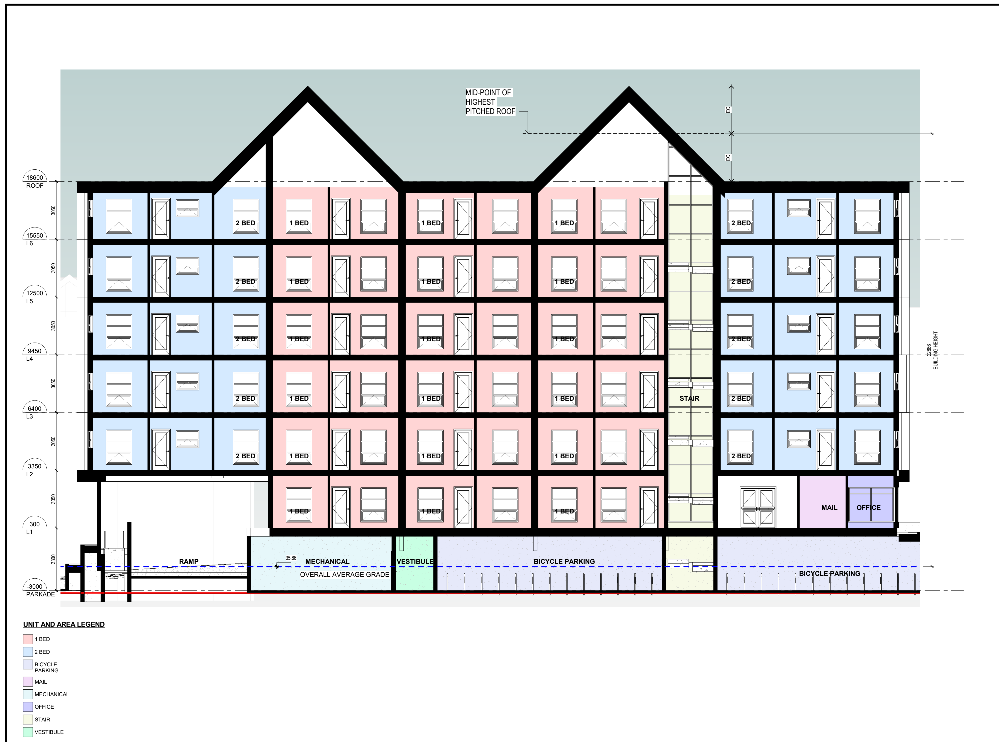
1 | APARTMENT BUILDING SECTION 1 1 : 100
