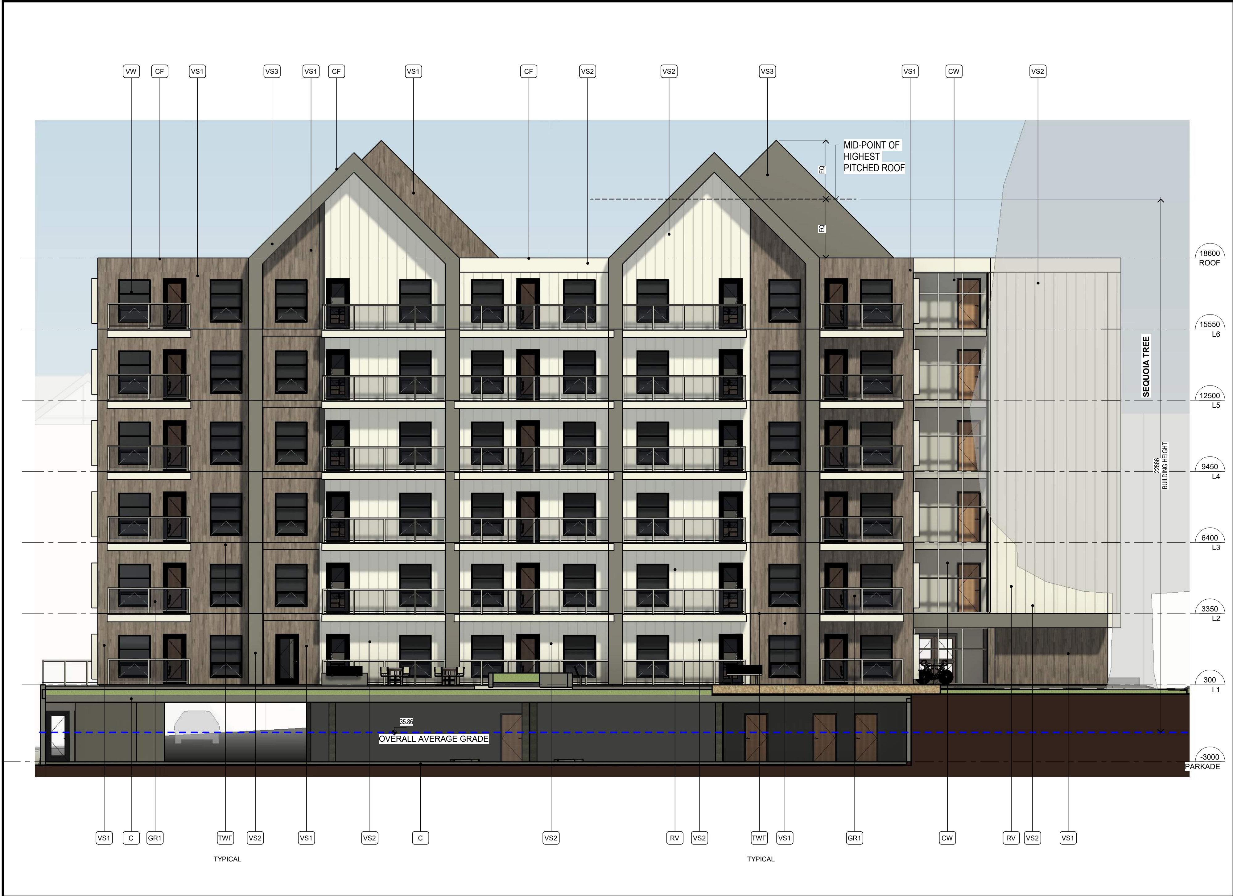
1 NORTH ELEVATION APARTMENT 1:100
