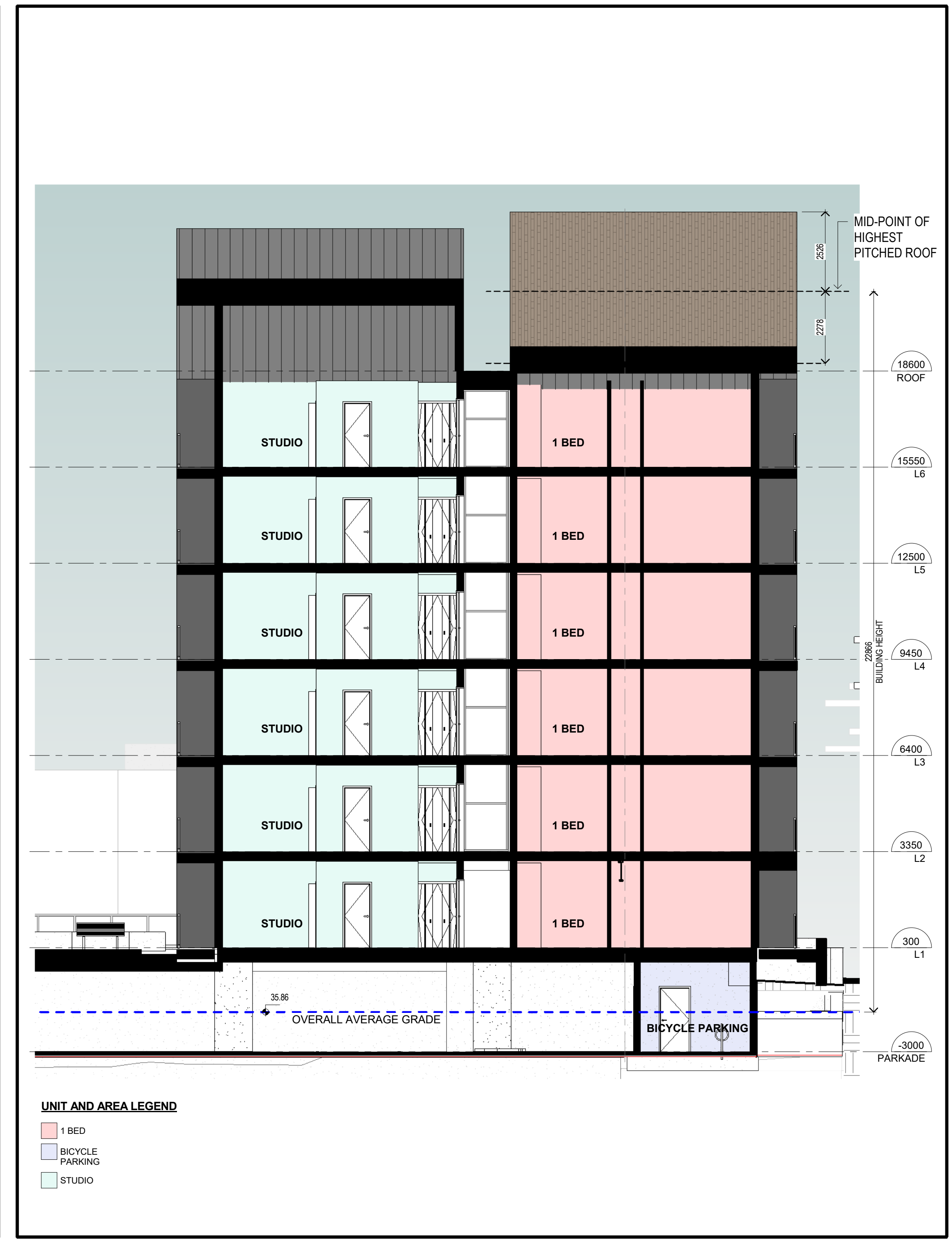
2 | APARTMENT BUILDING SECTION 4 1 : 100 VISUAL SCALE 1:100 @ Arch D
