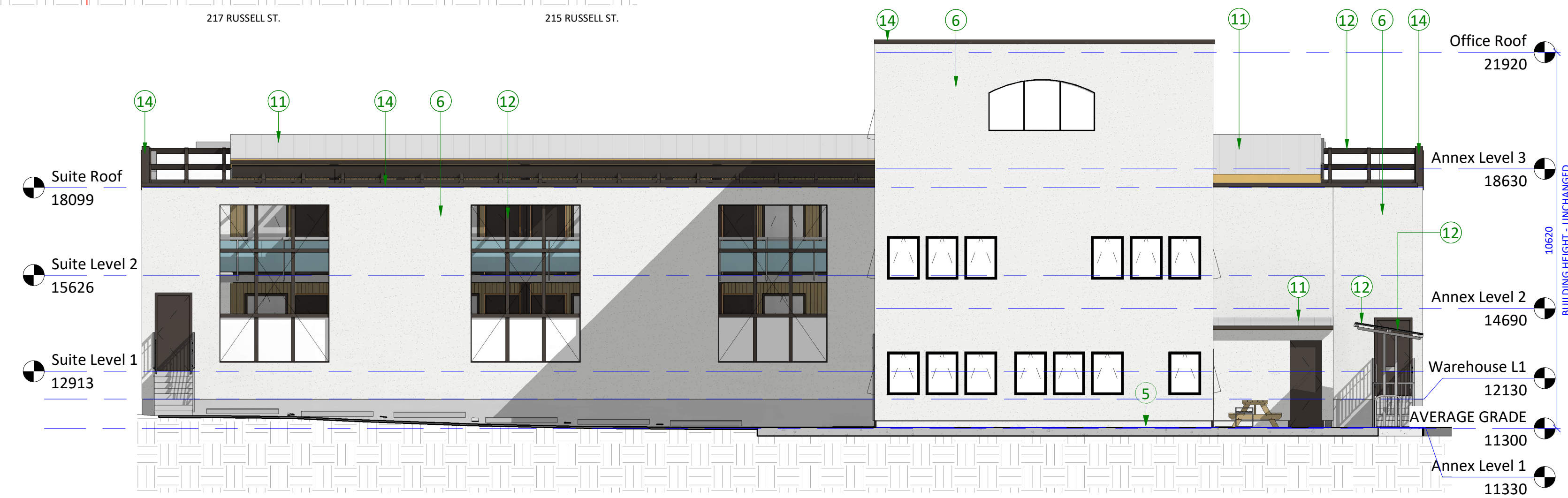
7 West Elevation - Shell 1:100
