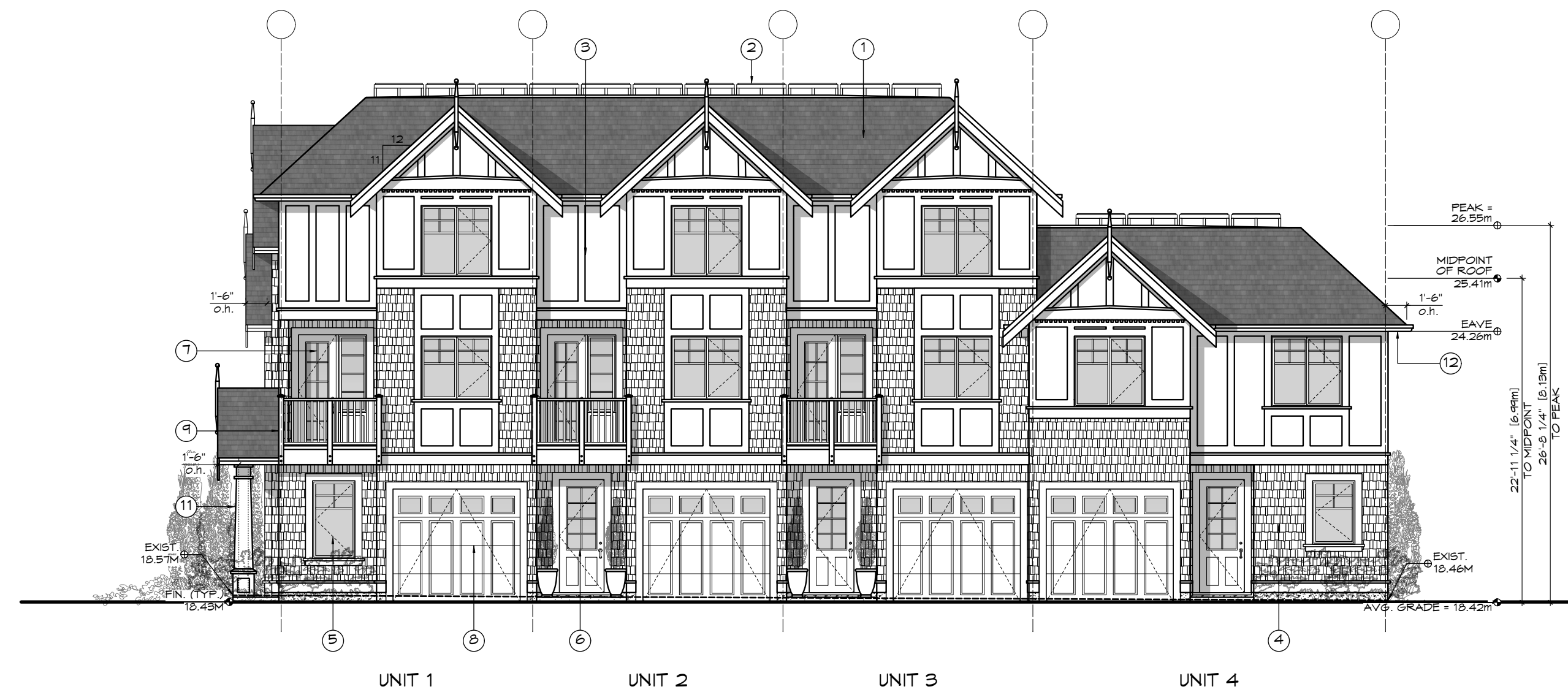
2 Side (Drive-aisle) Elevation - Bldg A Scale: 1:100
