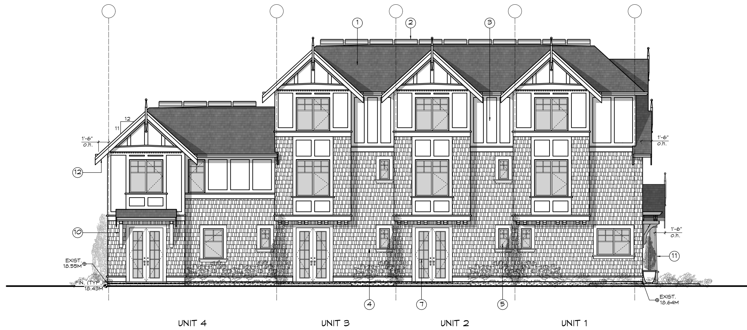
4 Side (S) Elevation - Bldg A Scale: 1:100
