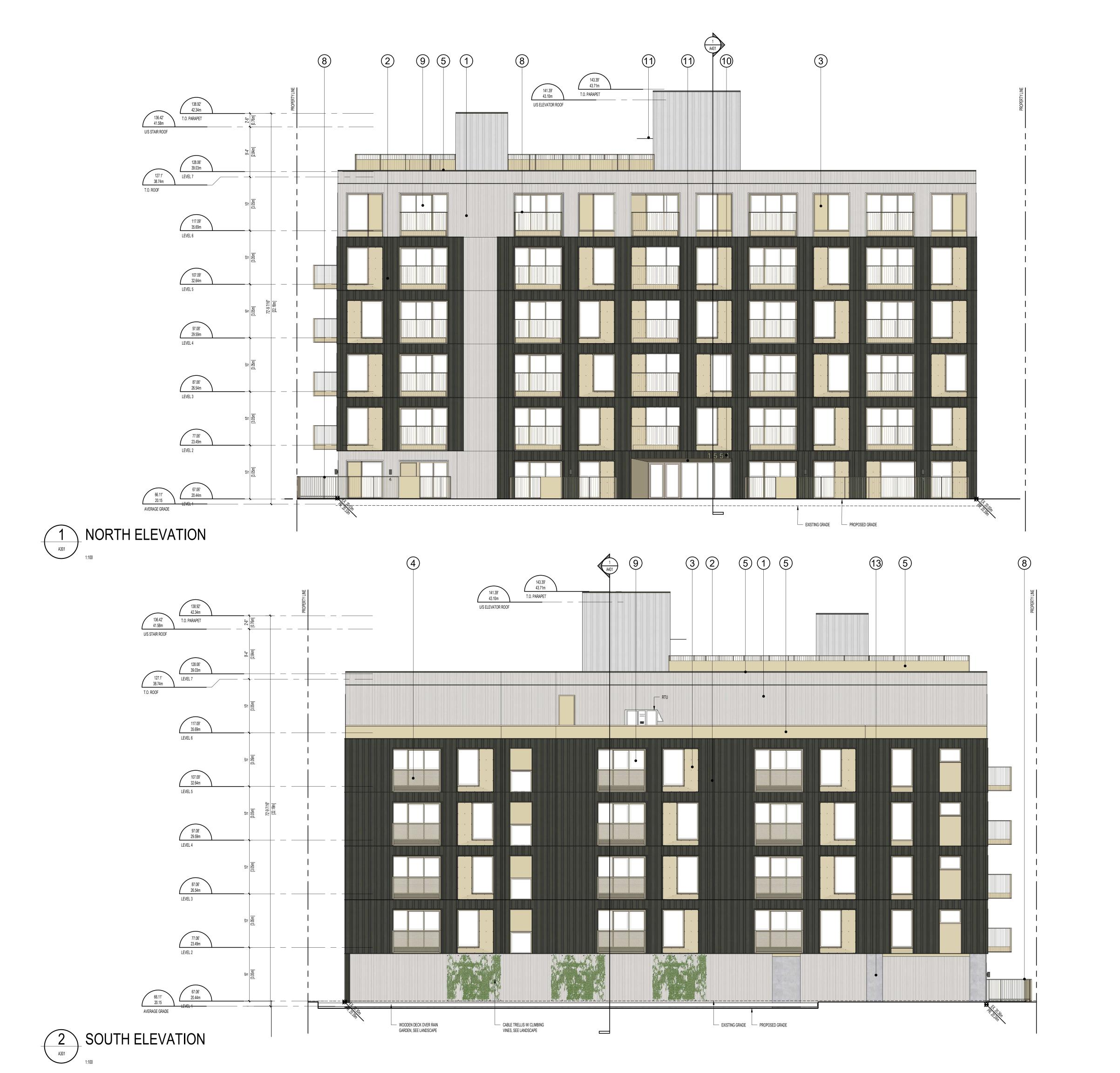
CERACLAD 8" REVEAL . 12" BOX RIB METAL PANEL (W/ 2" EXT INSULATION) 3. 4 GA. FACE MOUNTED METAL PANEL
