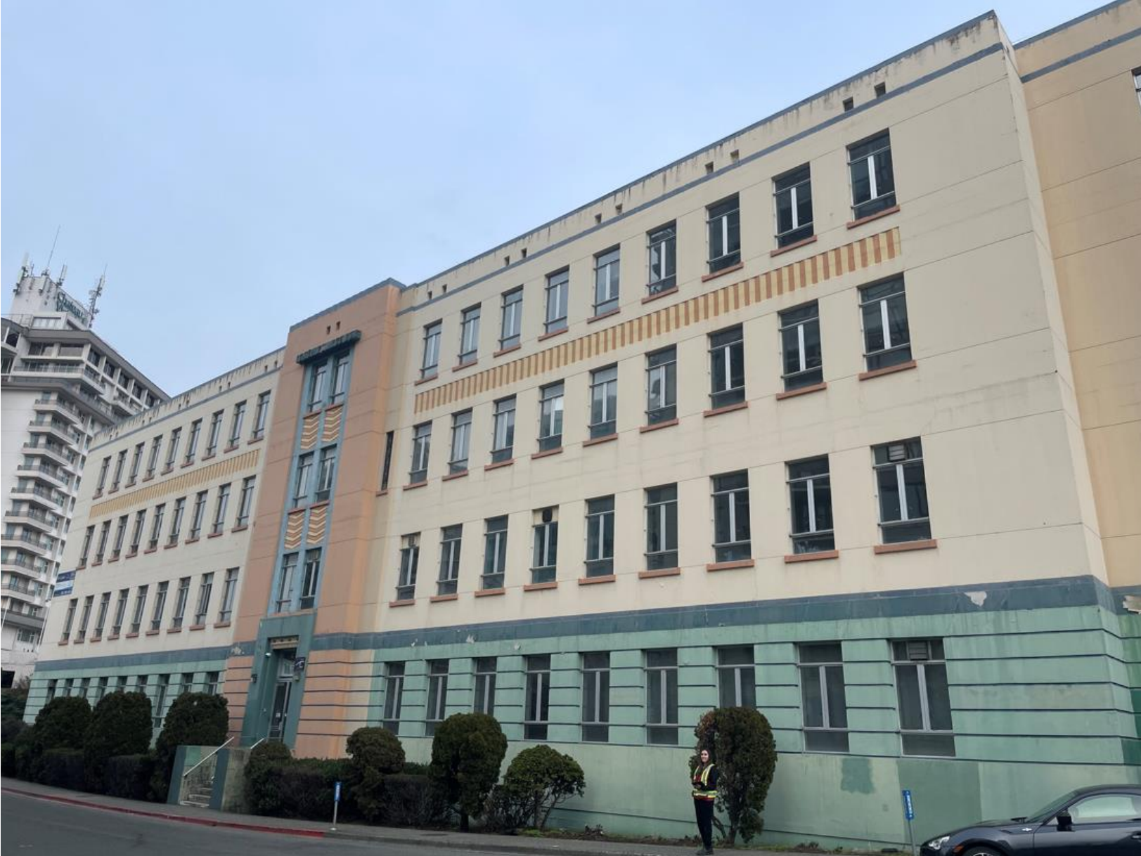
Above and below: Fixed and operable single glazed window units set within metal frames in punched openings.
