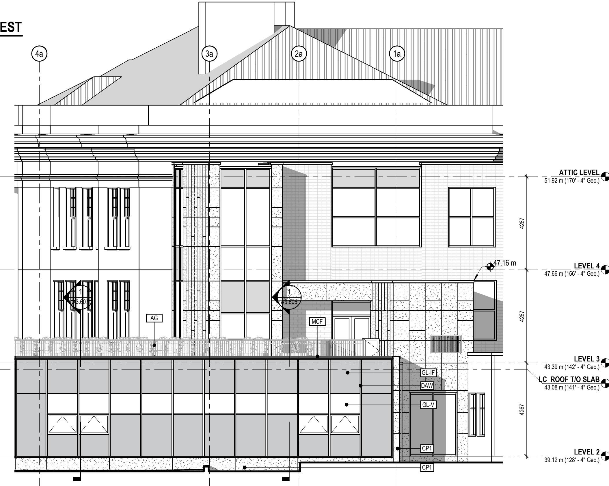
5 ELEVATION - NLC - NORTH 1 A3.311 1:100
