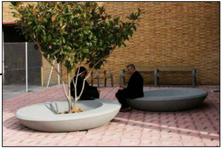
White Concrete Oval Planters with 5' x 2' Soil Depth. Seating lip 1.5' to 2'.5'
