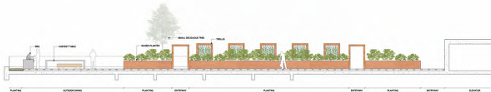
2 SECTION THROUGH ROOF AMENITY LOOKING NORTH Scale: 1/8" = 1'-0"
