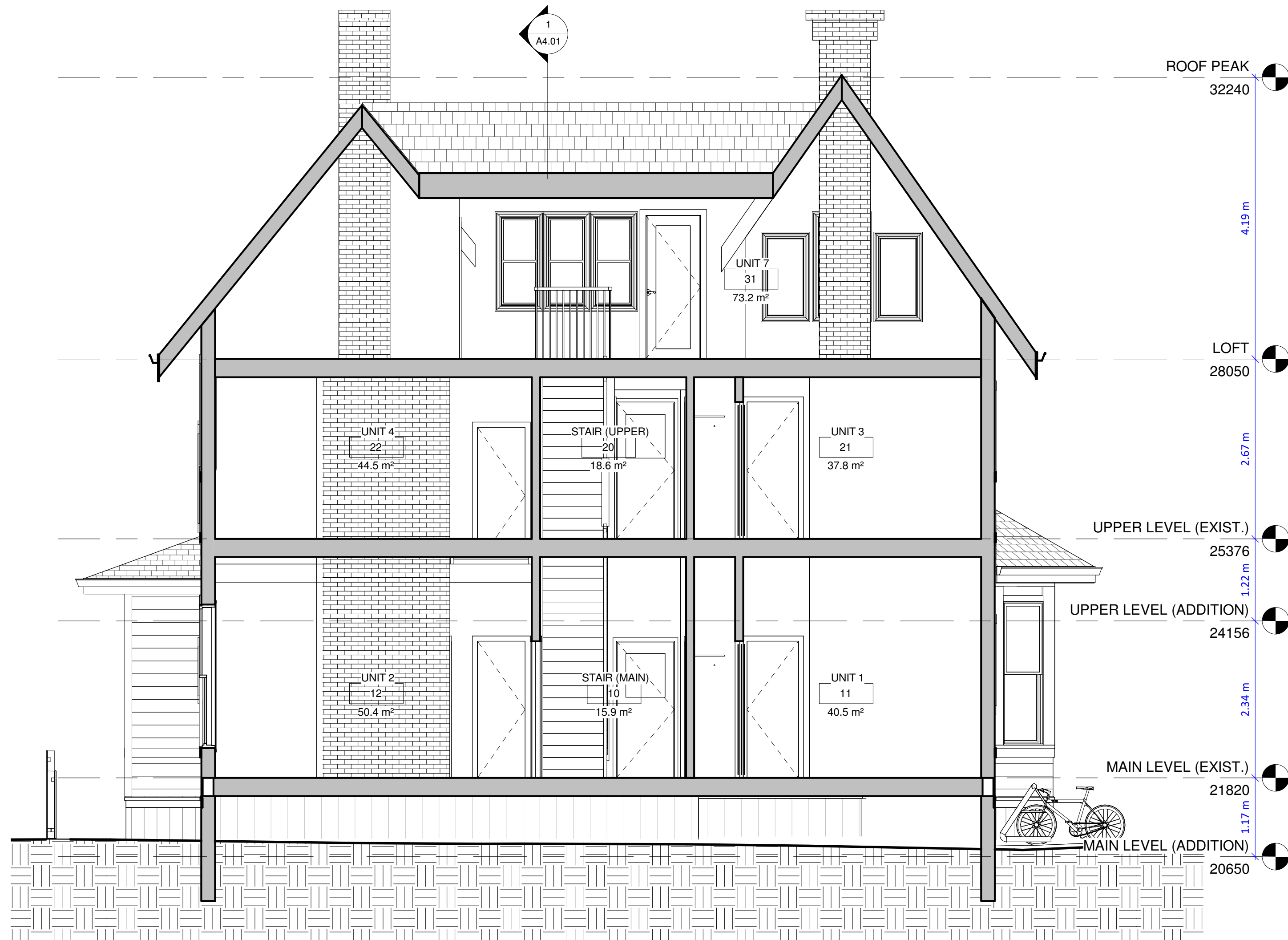
2 BUILDING SECTION - E/W (FACING S) @ EXISTING HOUSE 1 : 50
