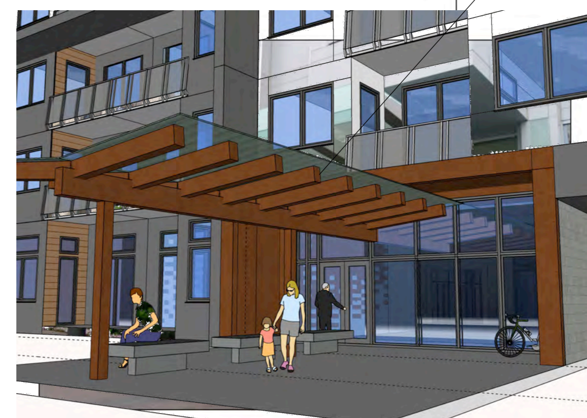
Heavy Timber and Glass Entrance Canopy
