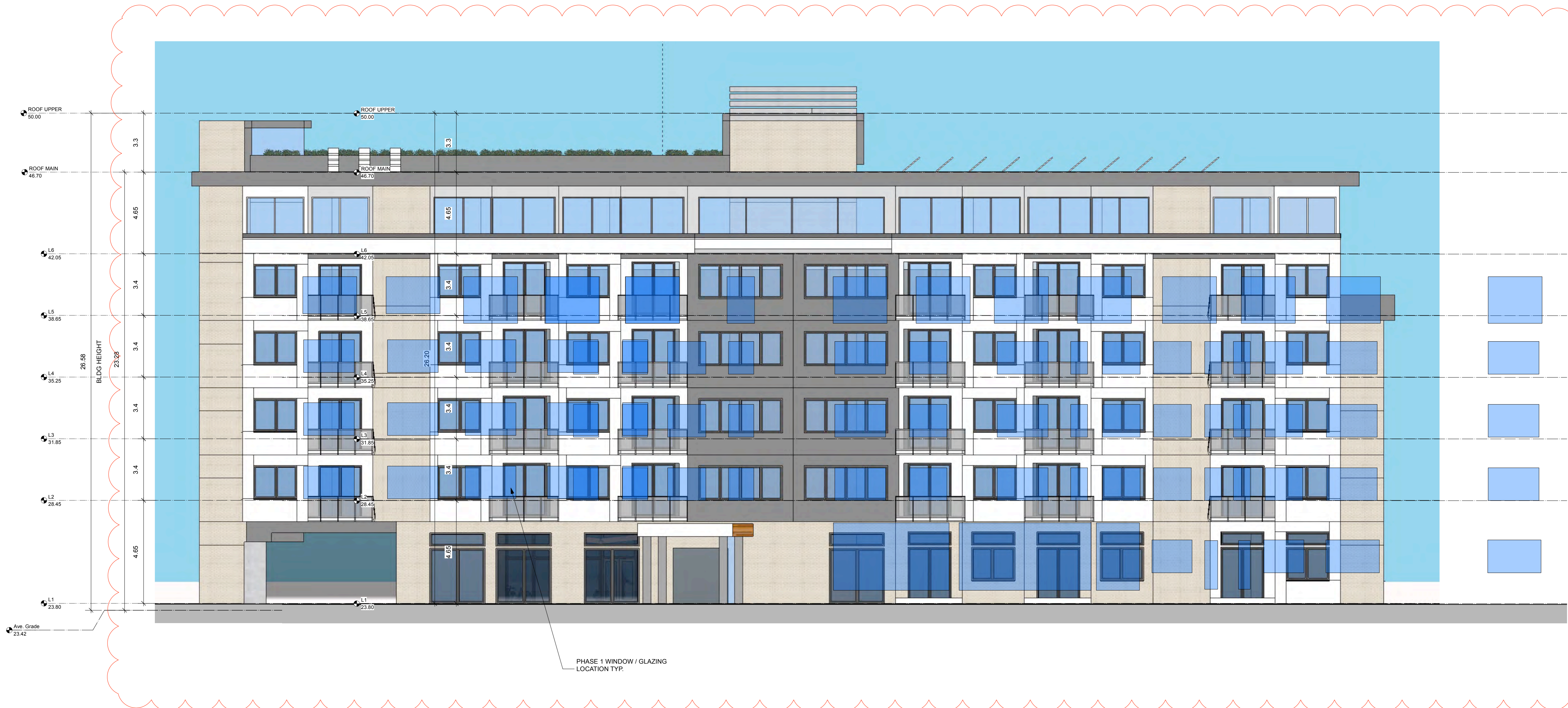
EAST ELEVATION WITH PHASE 1 WINDOW OPENINGS OVERLAID
