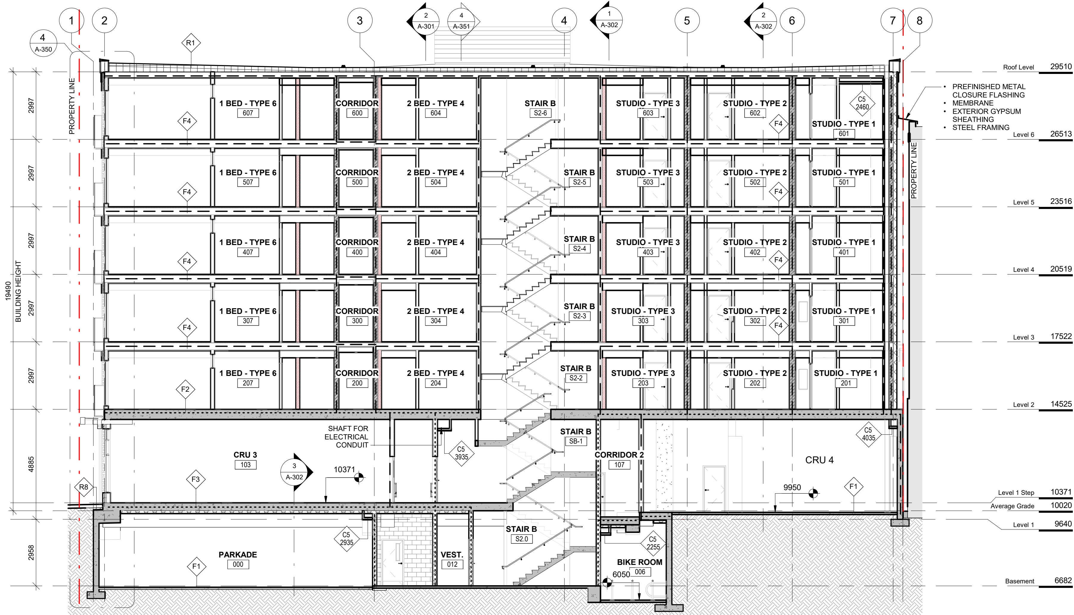
2 Building Section EW 2 - Looking North SCALE = 1 : 100
