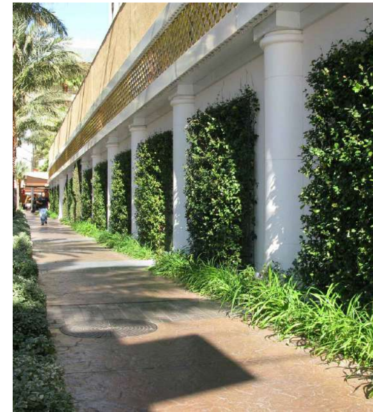
EAST SIDE, PARKADE WALL: WALLMOUNTED GREEN WALL PANELS GREENSCREEN 'ELEMENTS' MODULAR PANELS CUSTOM SIZE TO FIT, MOUNT PER MANUFACTURER SPECIFICATION
