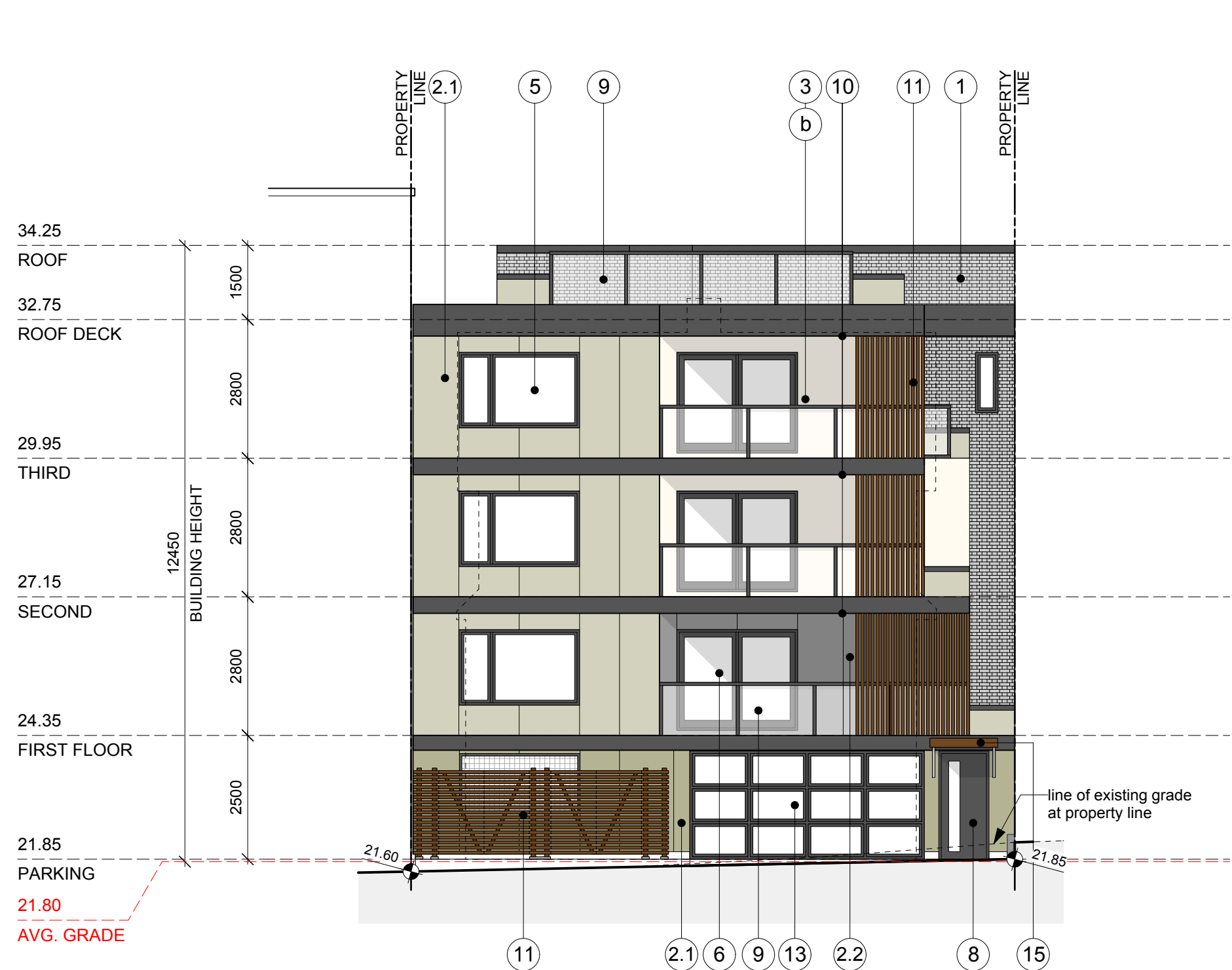
1 MEARES STREET (REAR) SOUTH ELEVATION Scale: 1:100
