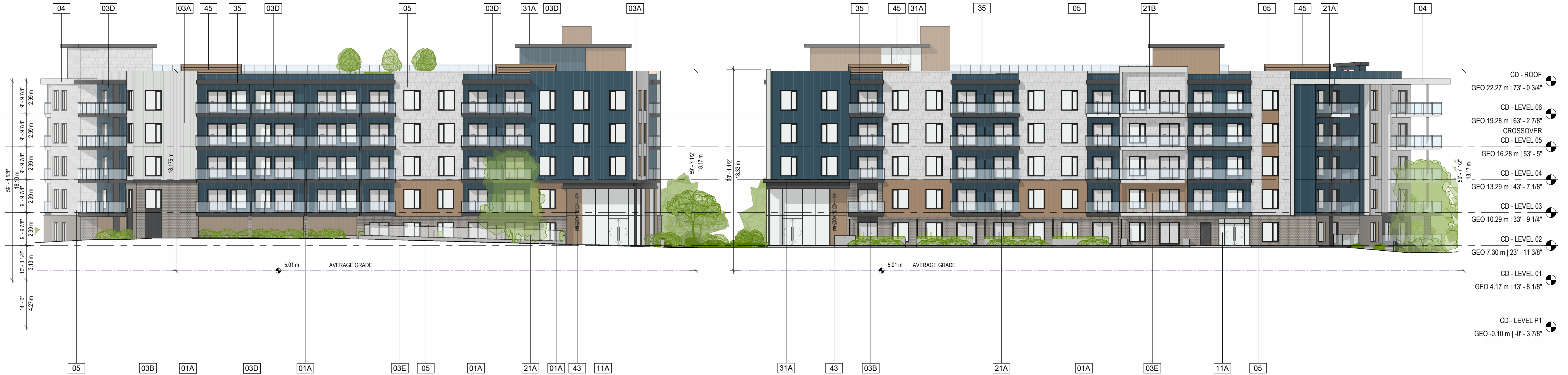
2 BLDG C + D NORTH ELEVATION DP2.30.01 SCALE: 1/16" = 1'-0"
