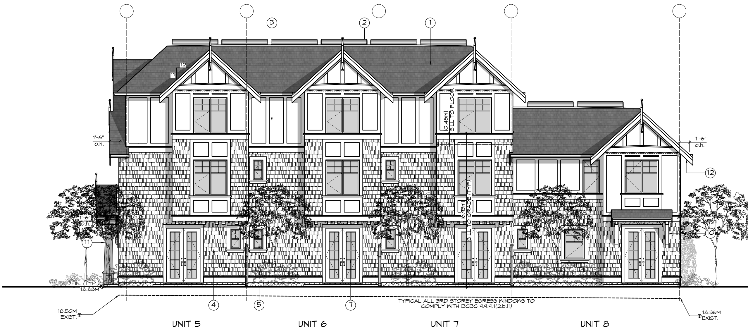
4 Side (N) Elevation - Bldg B Scale: 1:100
