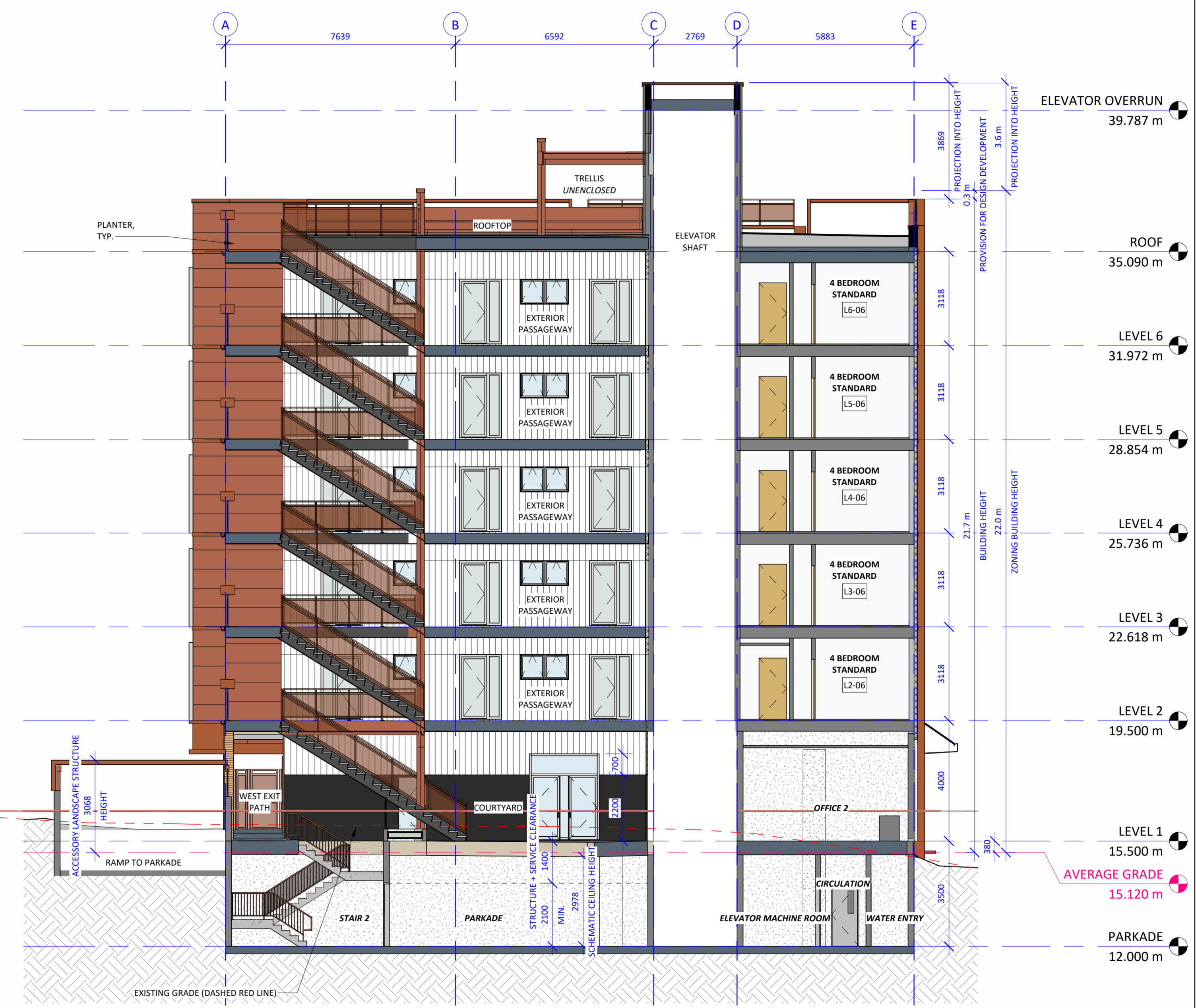
② NORTH-SOUTH SECTION THROUGH ELEVATOR 1 : 100
