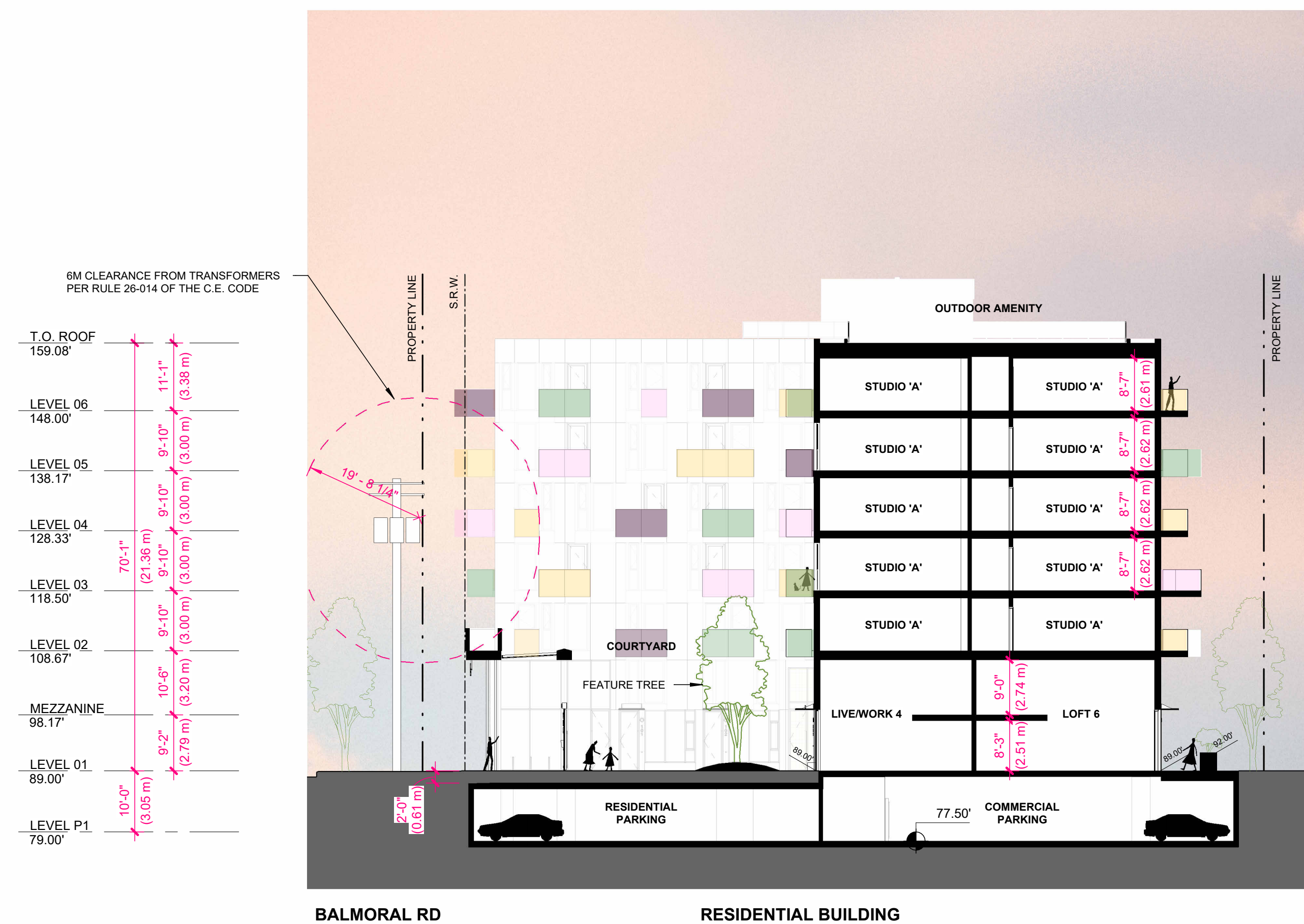
2 SITE SECTION THROUGH RESIDENTIAL COURTYARD LOOKING WEST
