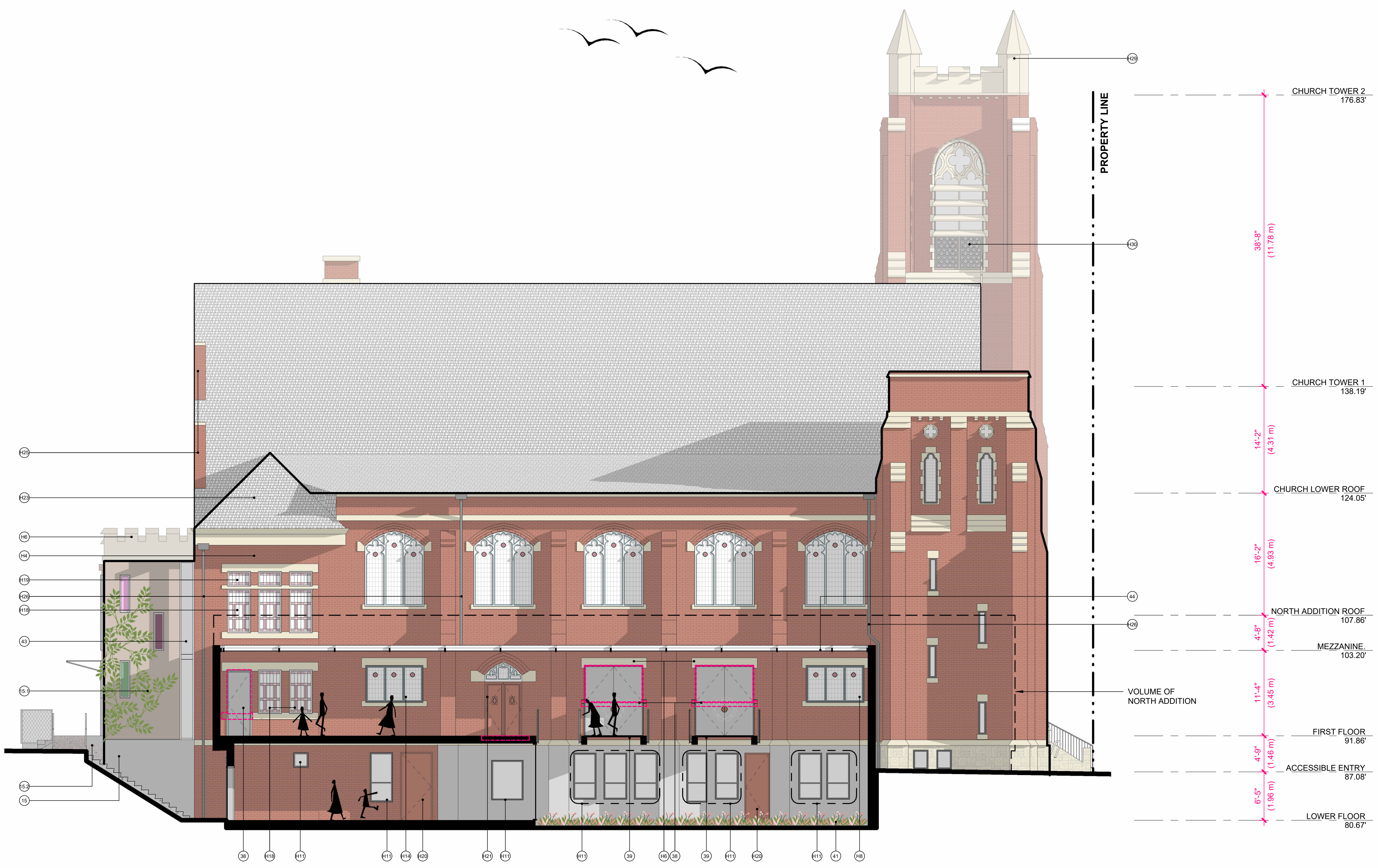
1 NORTH ELEVATION AT CHURCH 1/8" = 1'-0"
