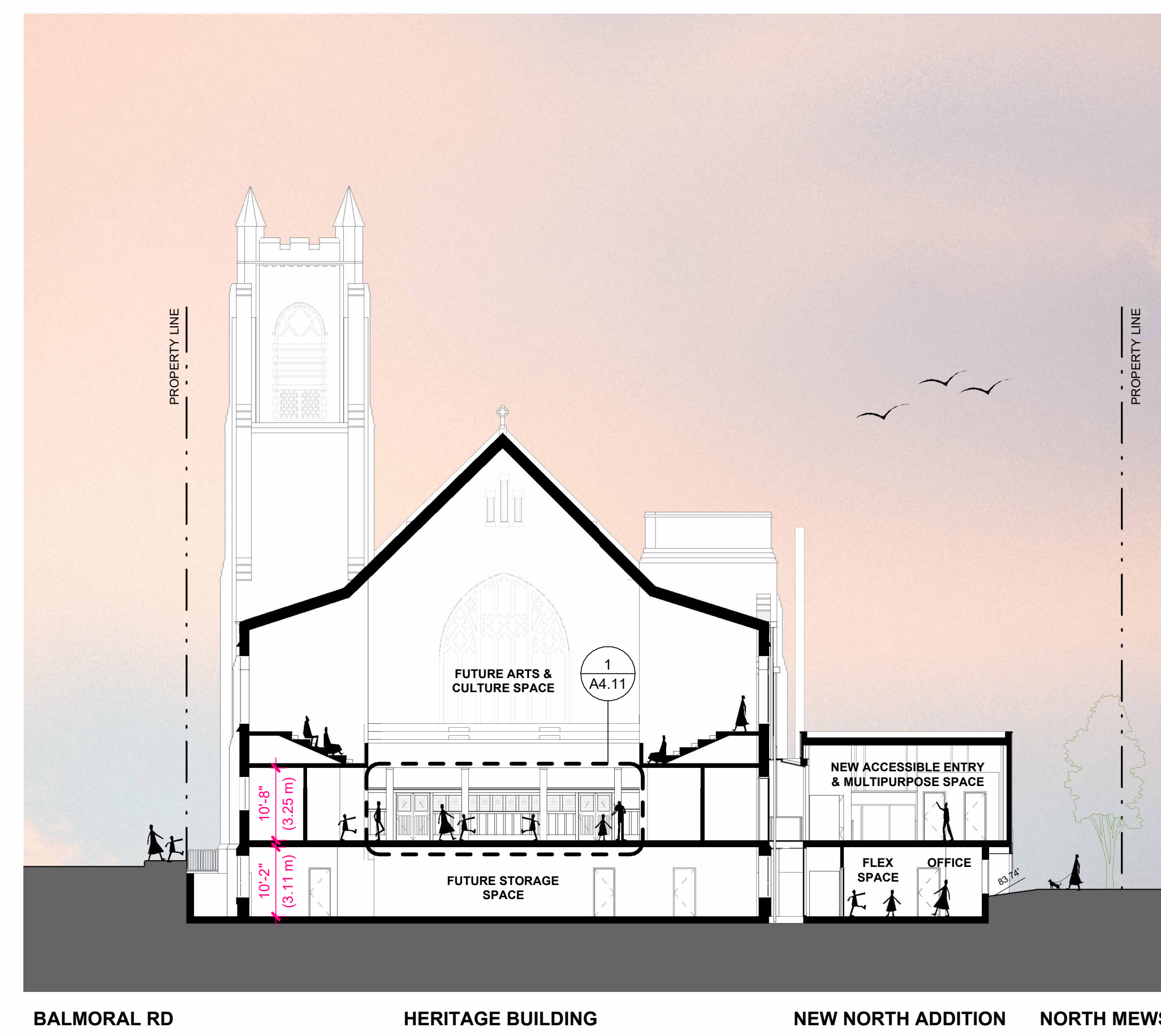
4 SITE SECTION THROUGH HERITAGE BUILDING LOOKING WEST
