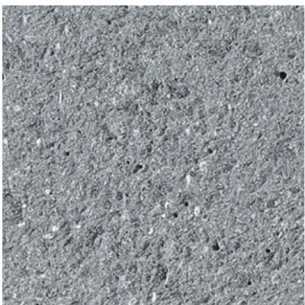
CR1 CR2 EXPOSED CONCRETE SANDBLASTED
