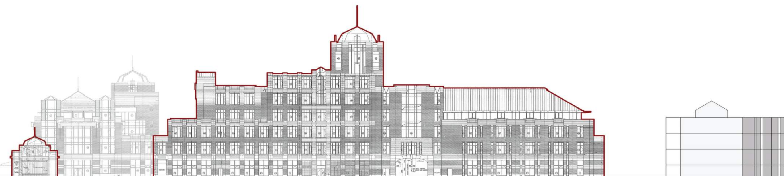
AN ILLUSTRATIVE 1996 VICTORIA ACCORD PROPOSAL (APPROVED FOR BUILDING PERMIT) FOR A 6 STOREY 22M HIGH COMMERCIAL/OFFICE PROJECT IN COMPLIANCE WITH THE 1994 LEGISLATIVE PRECINCT BUILT FORM GUIDELINES
