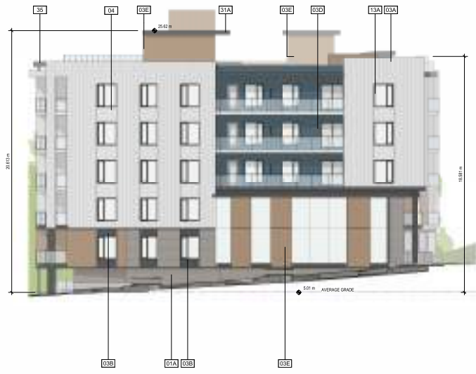
1 BLDG 2A EAST ELEVATION SCALE: 3/32" = 1'-0"
