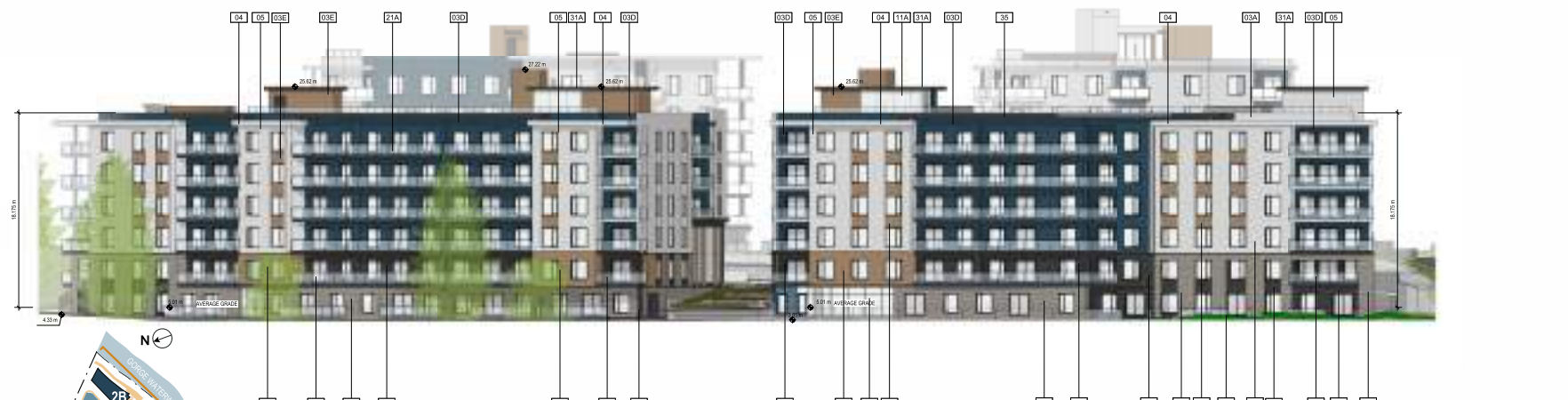
1 BLDG 2A/2B SOUTHEAST ELEVATION SCALE: 1/16" = 1'-0"
