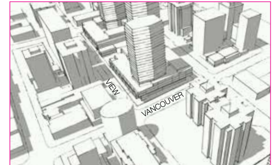
1. Bird's eye view looking north west. The podium massing steps down towards View, providing a transition from the wider and busier Yates to narrower and quieter View.
