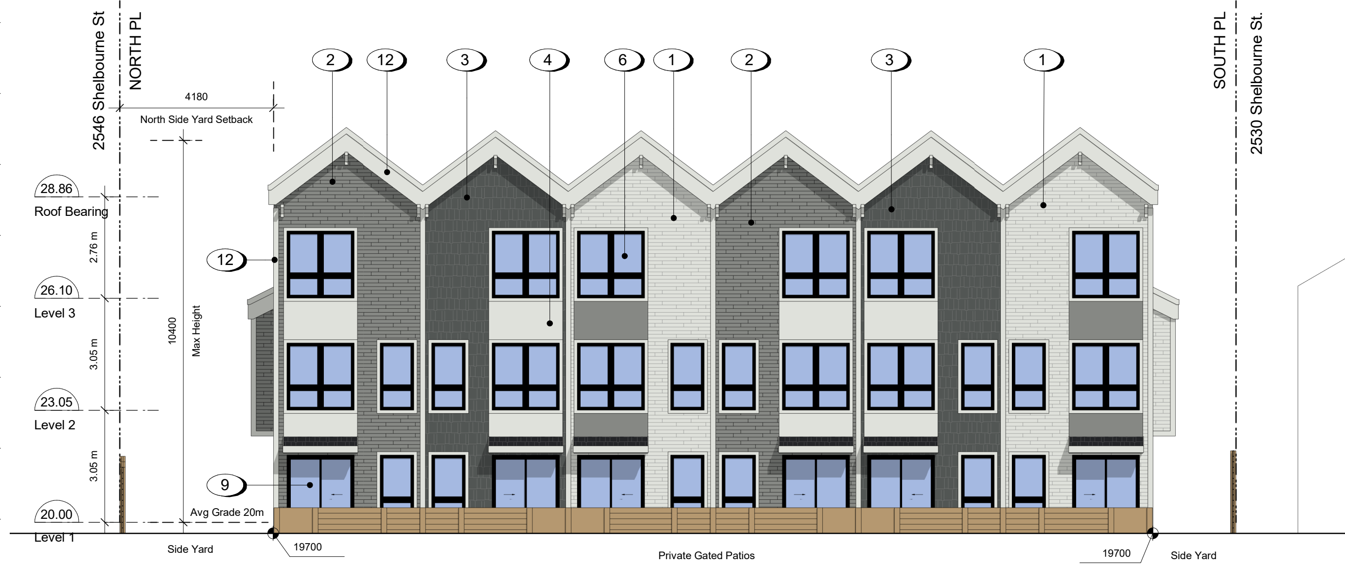
1 Rear Building - West Elevation A302 SCALE: 1 : 100
