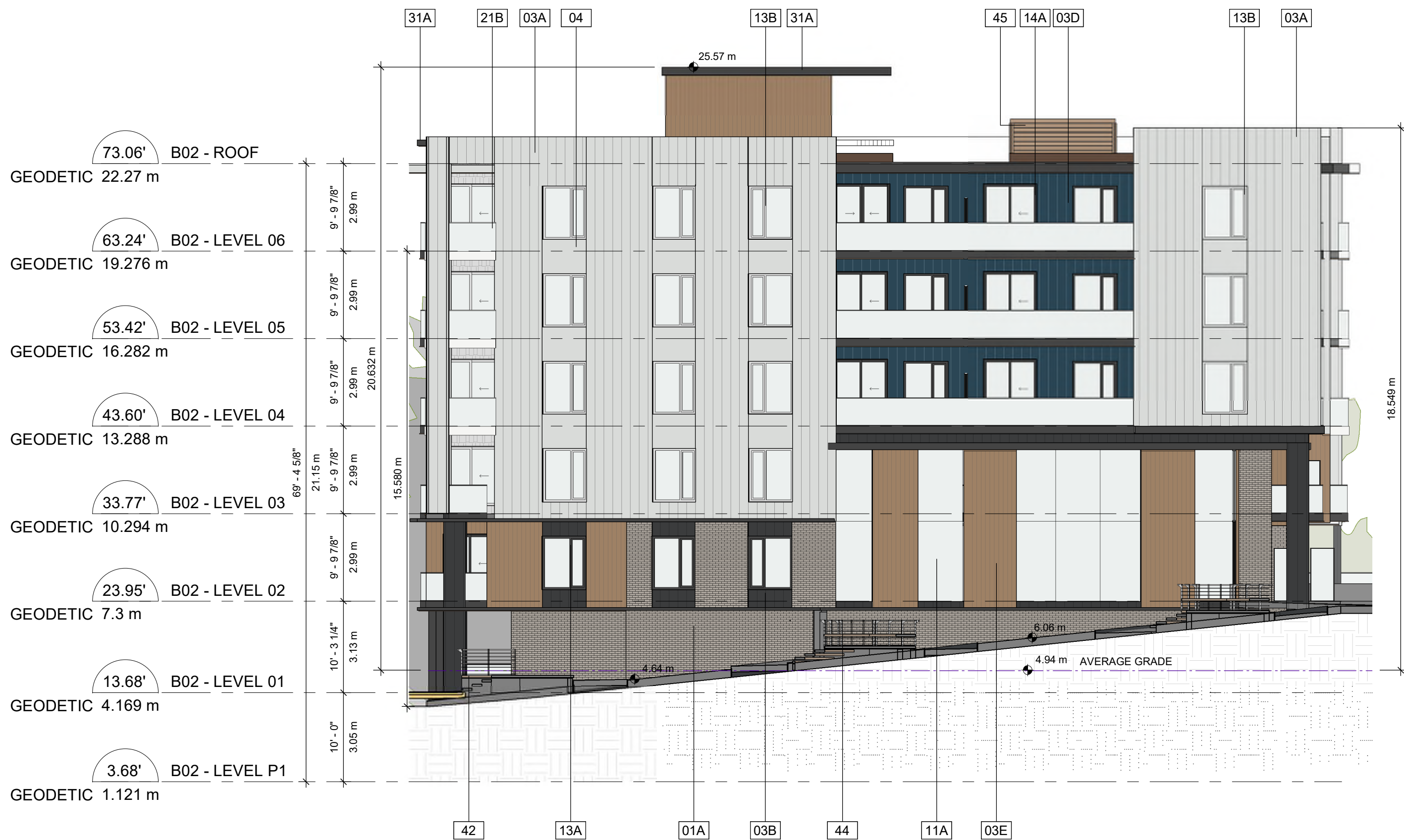
1 BLDG 2A EAST ELEVATION DP2.30.02 SCALE: 3/32" = 1'-0"
