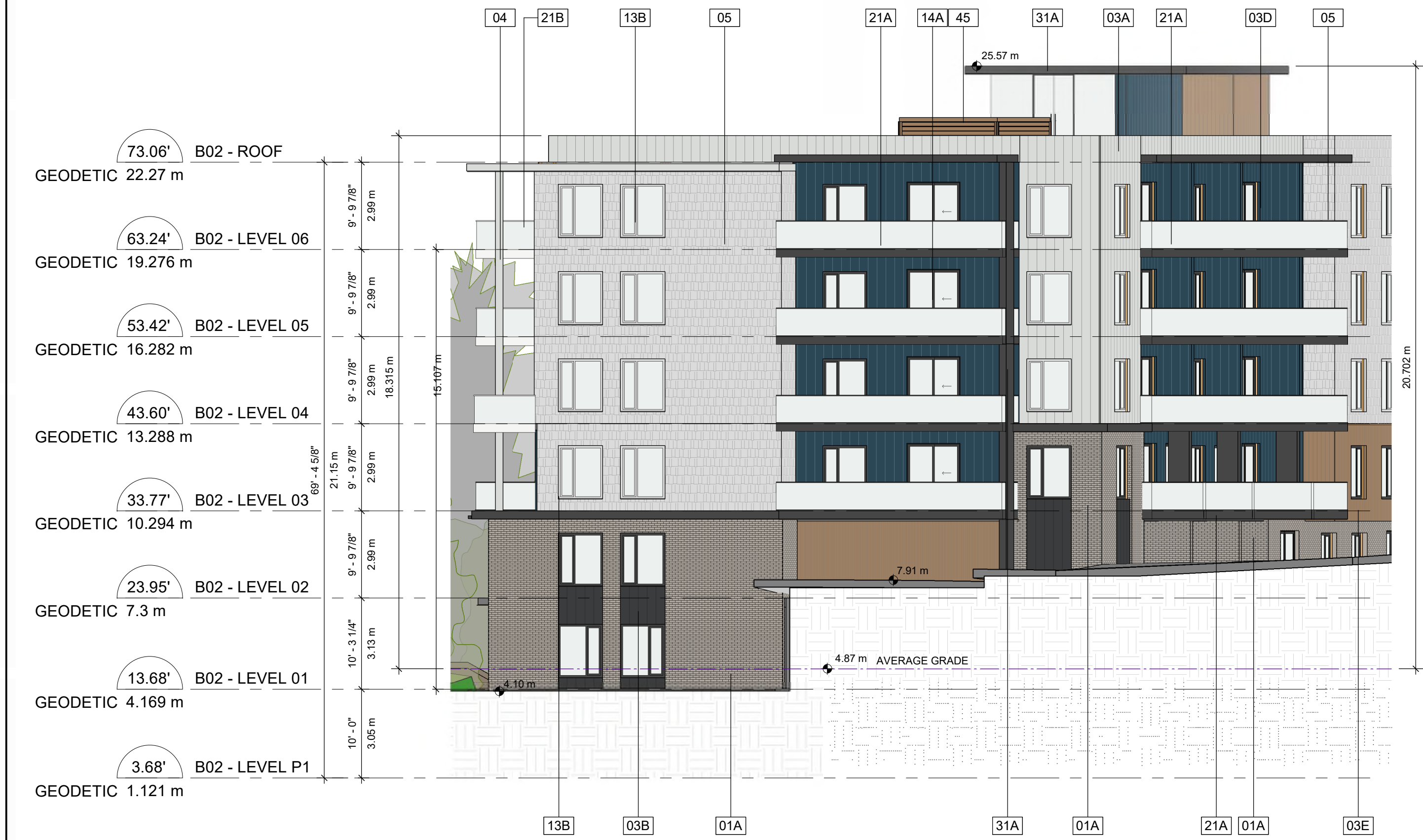
2 BLDG 2B NORTHEAST ELEVATION DP2.30.03 SCALE: 3/32" = 1'-0"
