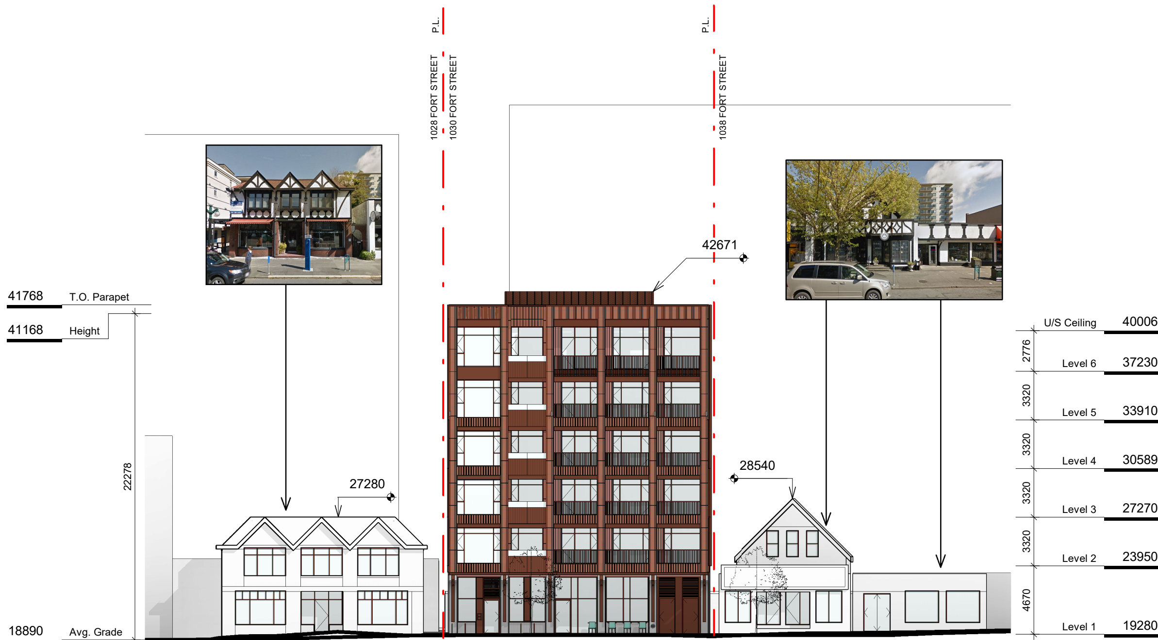
1 South Elevation - Fort Street Context SCALE = 1 : 250
