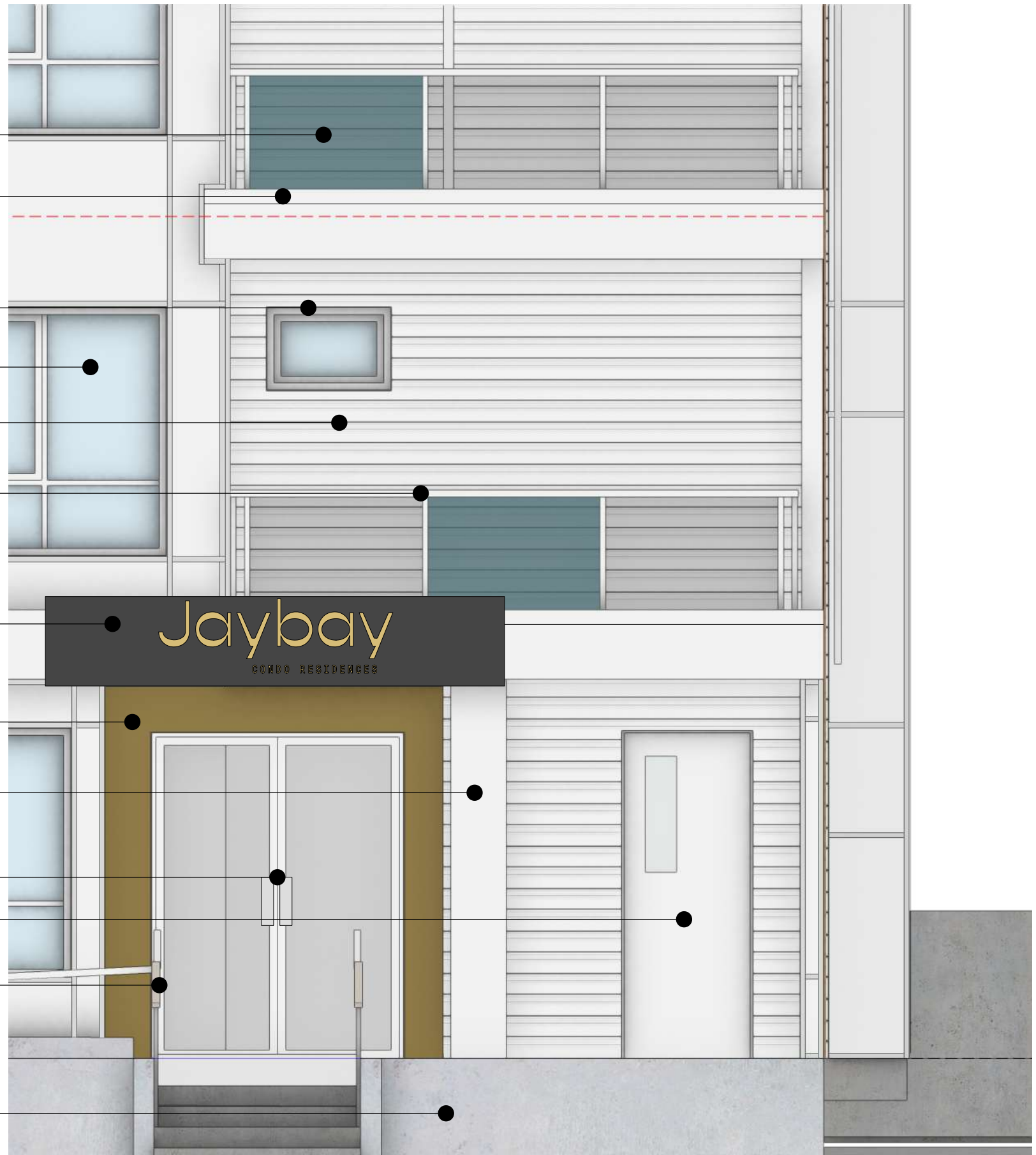
BALCONY RAILING CLEAR ANODIZED ALUMINUM FRAME WITH TEMPERED GLASS PANELS
