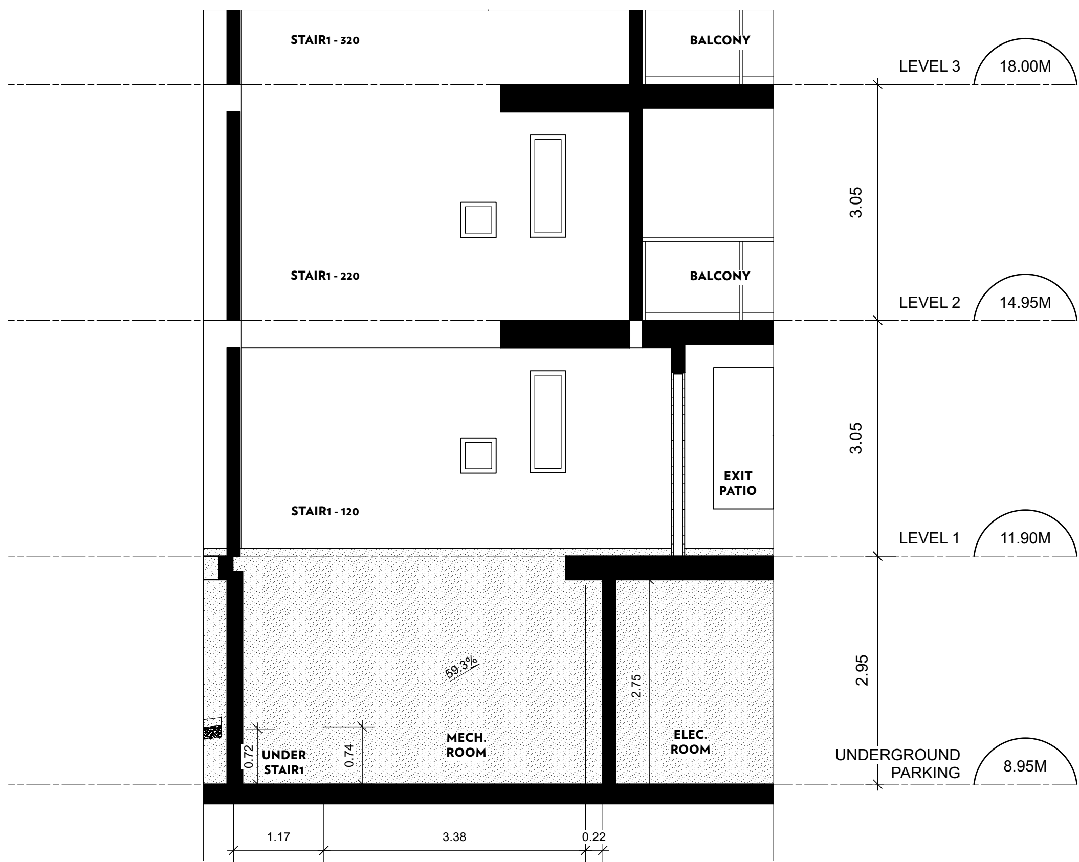
2 SECTION THROUGH MECH. ROOM Scale: 1:50
