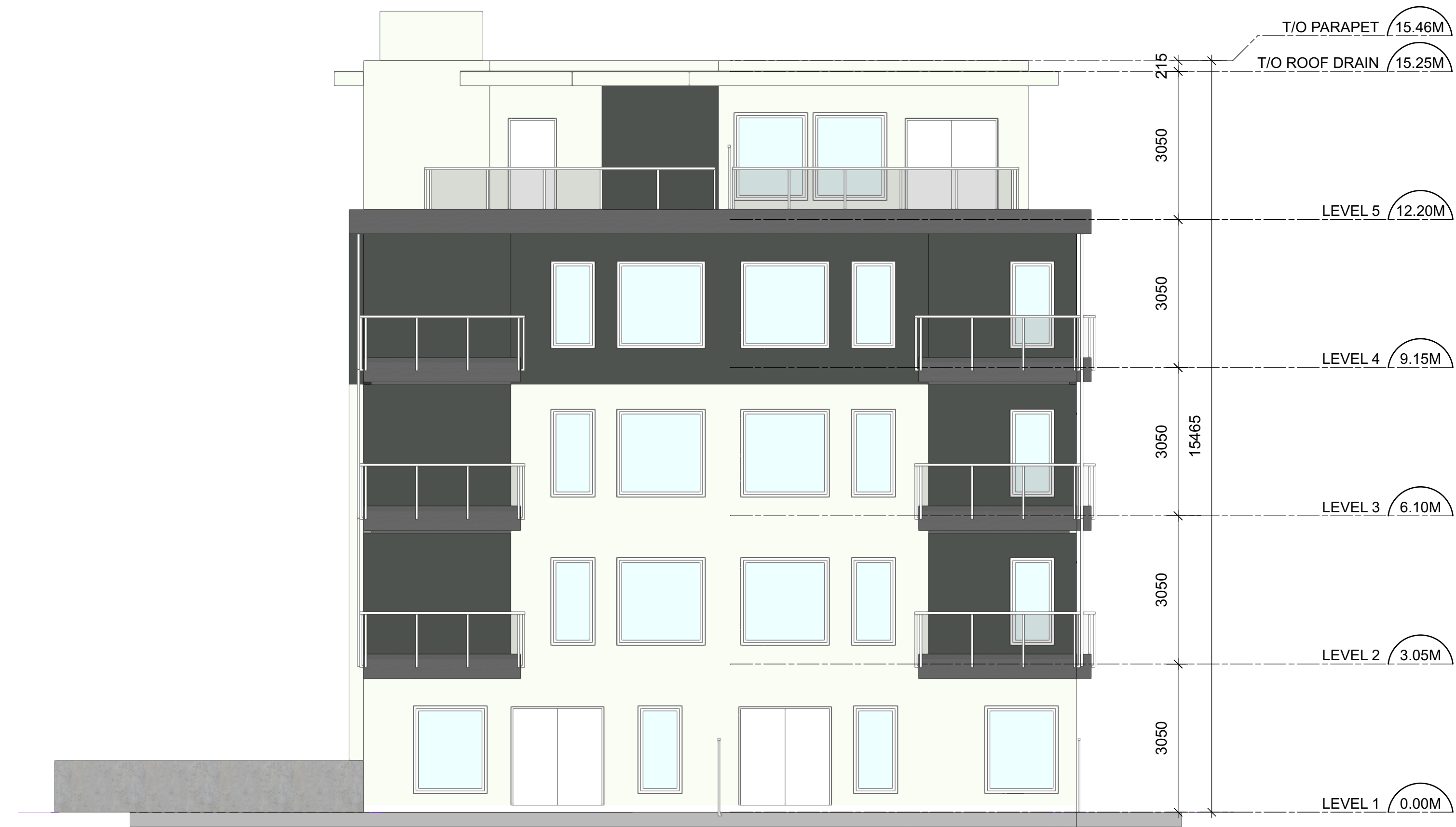
1 SOUTH ELEVATION - REAR FACADE Scale: 1:75
