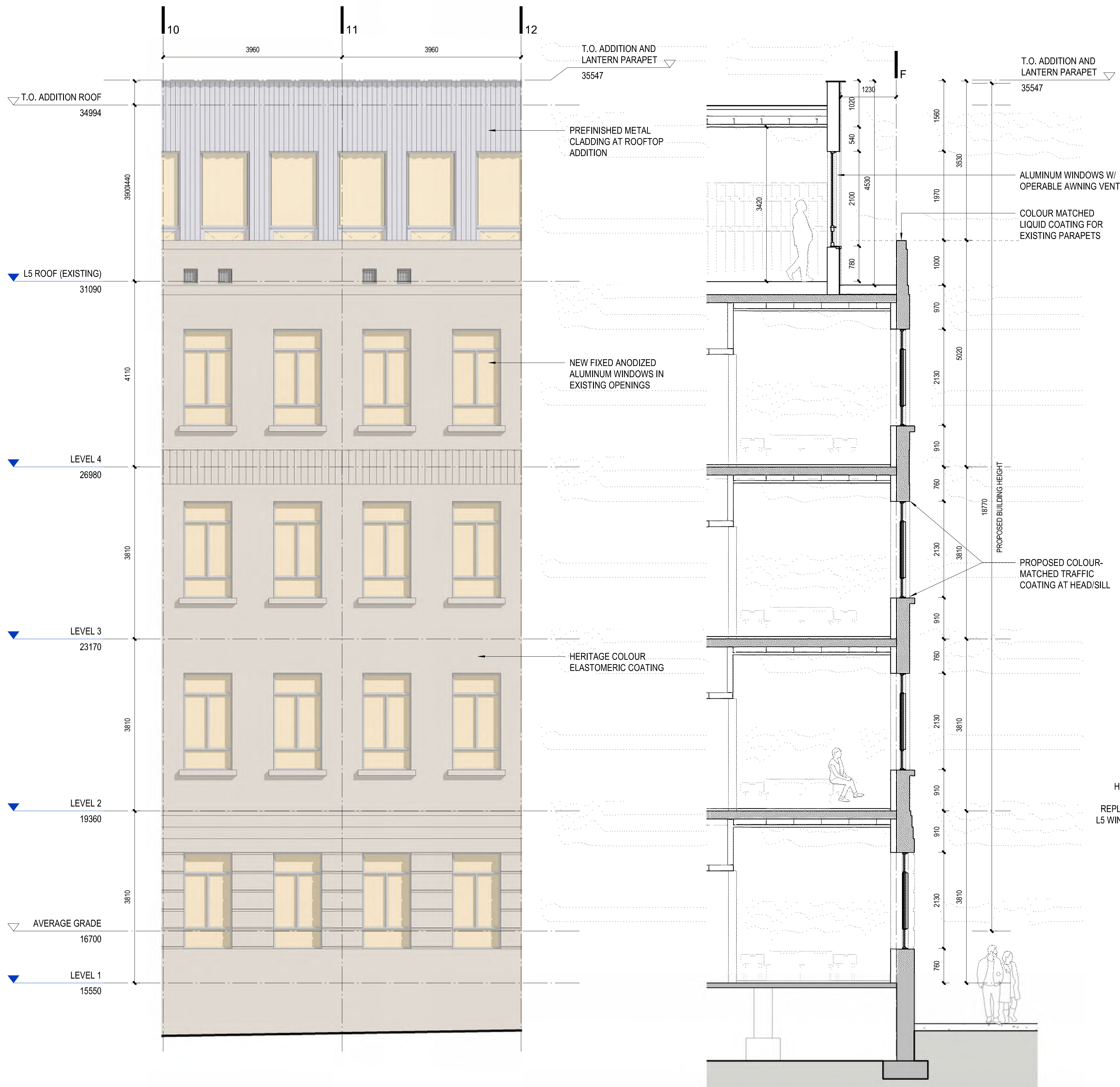
1 TYPICAL BAY - ELEVATION A204 1:50
