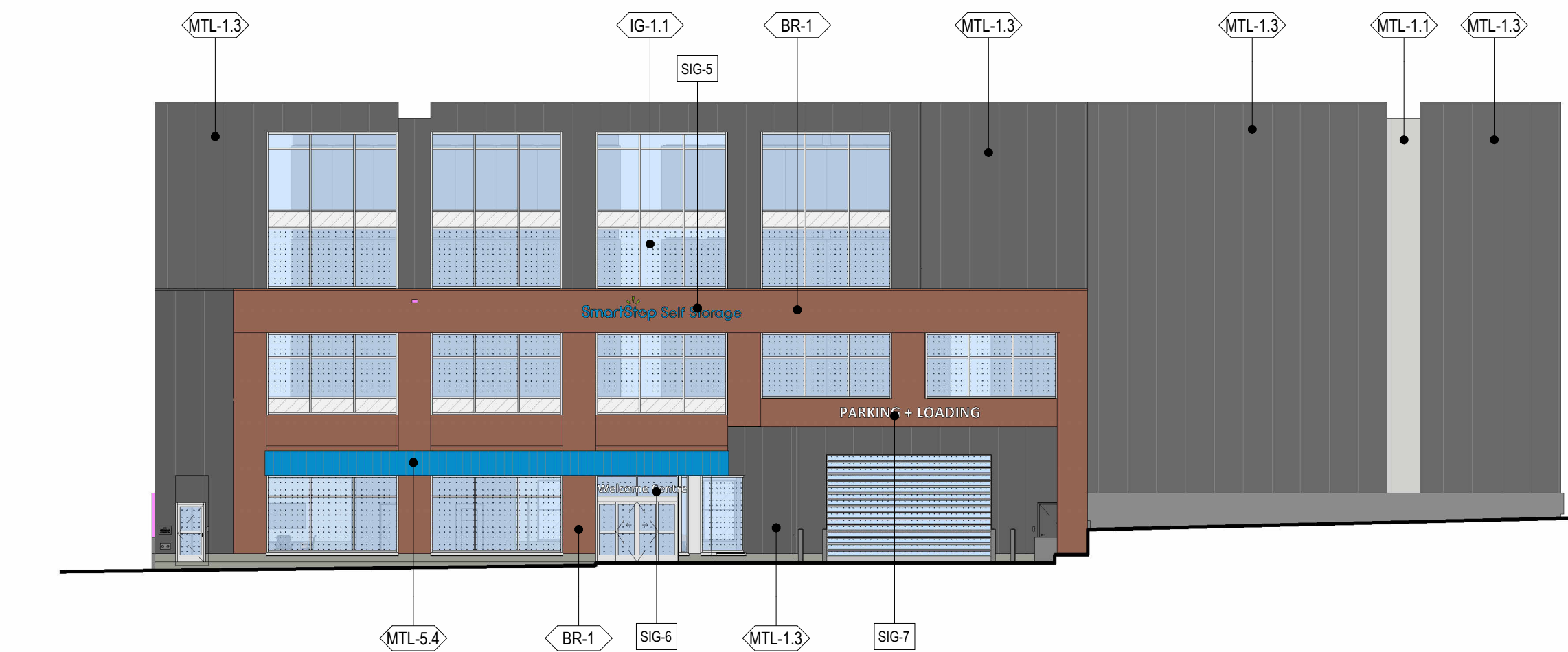
3 SOUTH ELEVATION EXTERIOR FINISHES A-210 1/16" = 1'-0"
