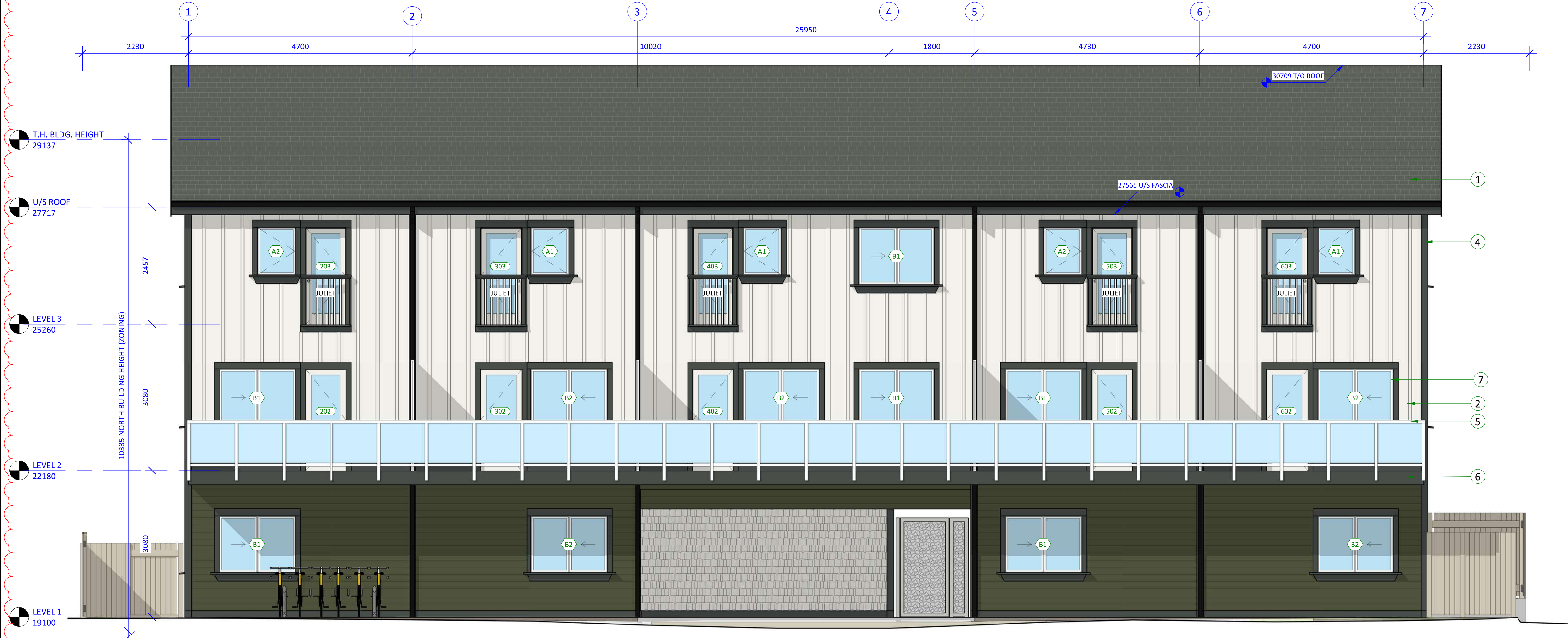
5 ELEVATION - SOUTH - NORTH BUILDING (LOT INTERIOR) A1.02 1 : 50
