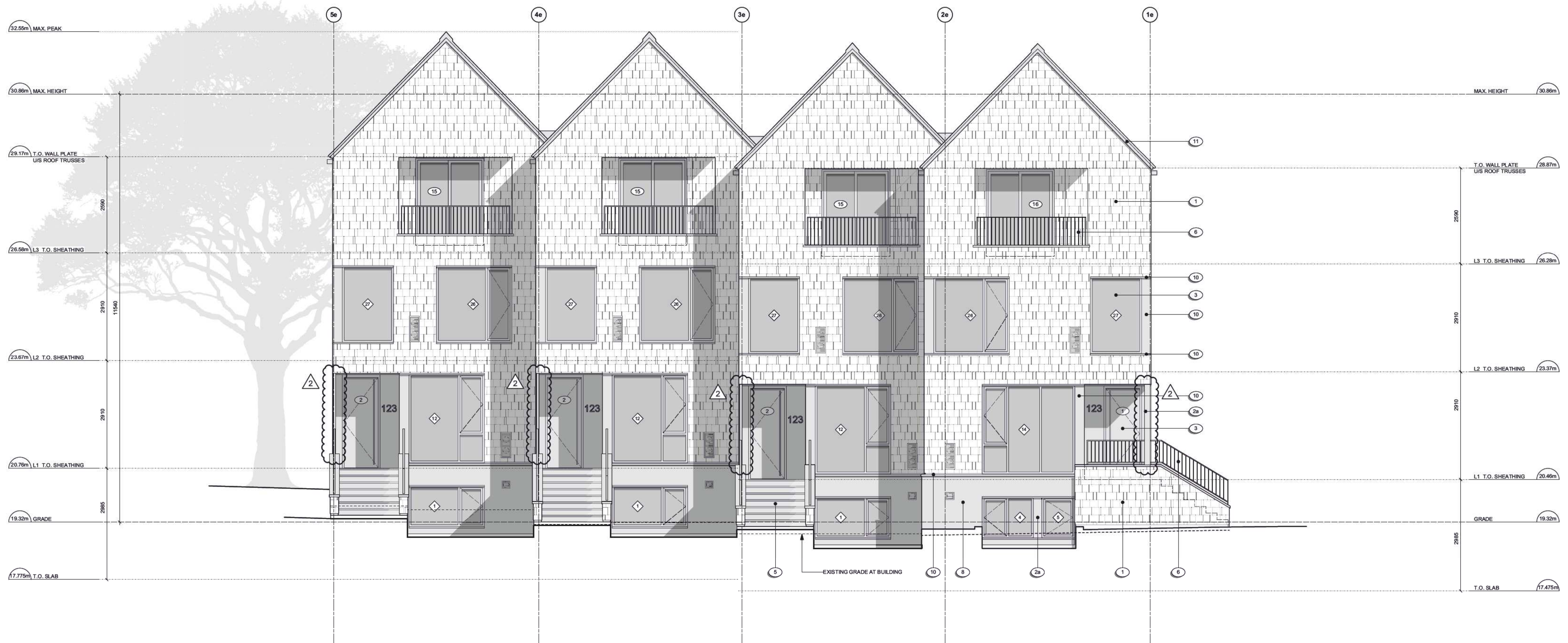
2 East Bldg. - West Elevation Scale: 1:50
