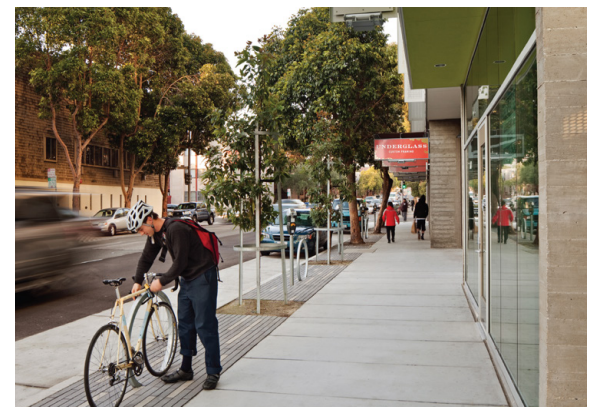
Bicycle parking area outside of clear sidewalk area; sidewalk paving extending beyond property line.
