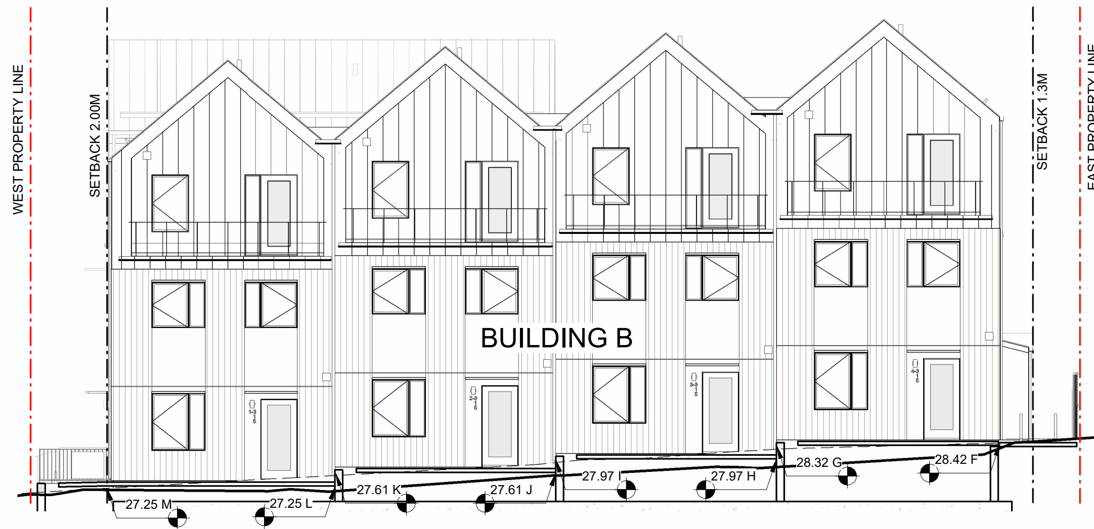
3 AVERAGE GRADE - SOUTH ELEVATION A.008 1:100
