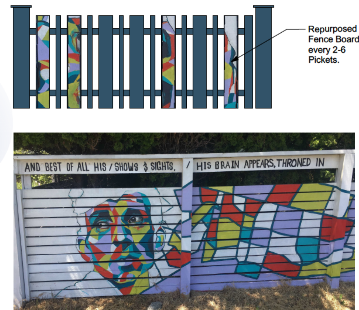
Proposed Picket Fence Detail
