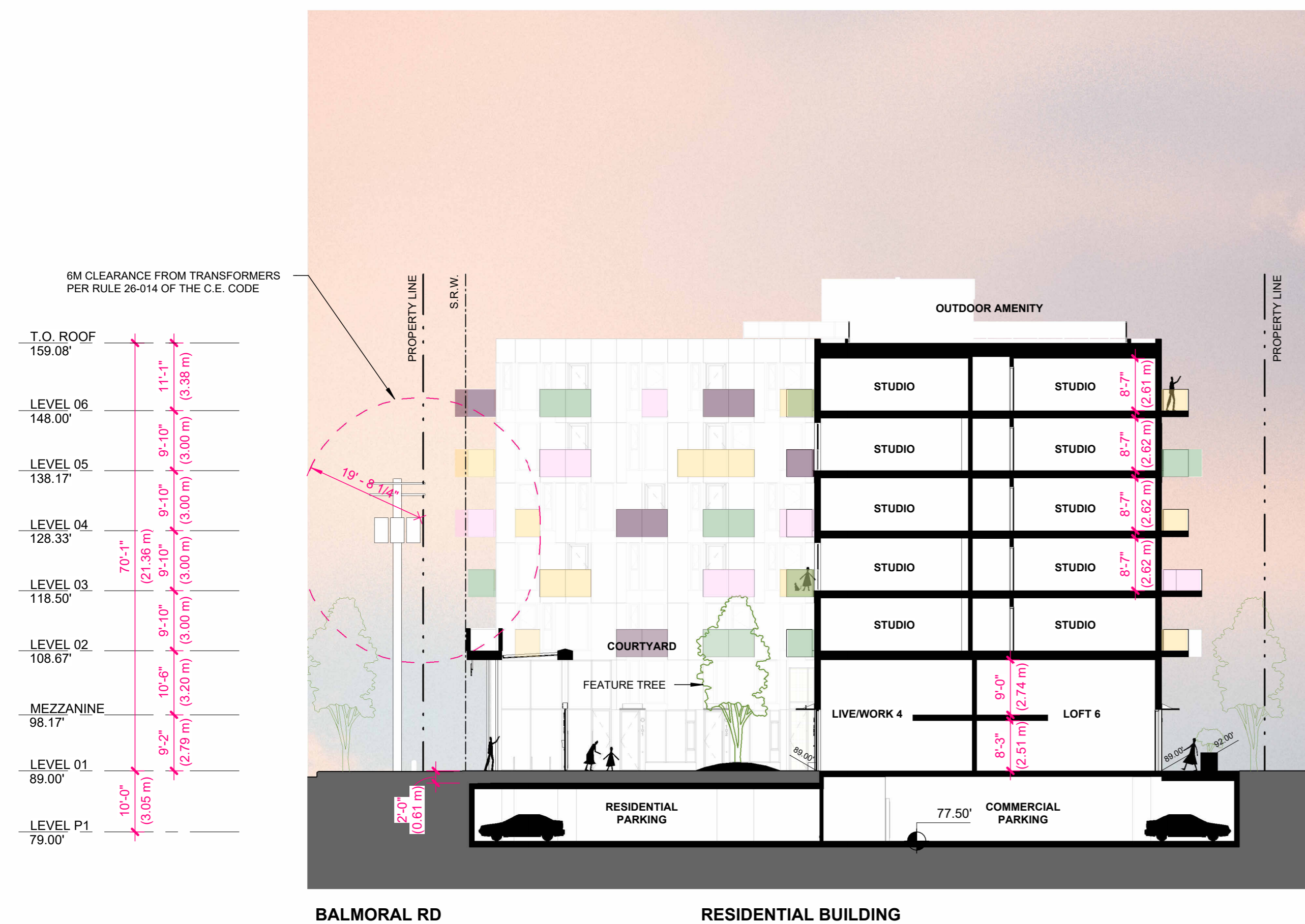
2 SITE SECTION THROUGH RESIDENTIAL COURTYARD LOOKING WEST
